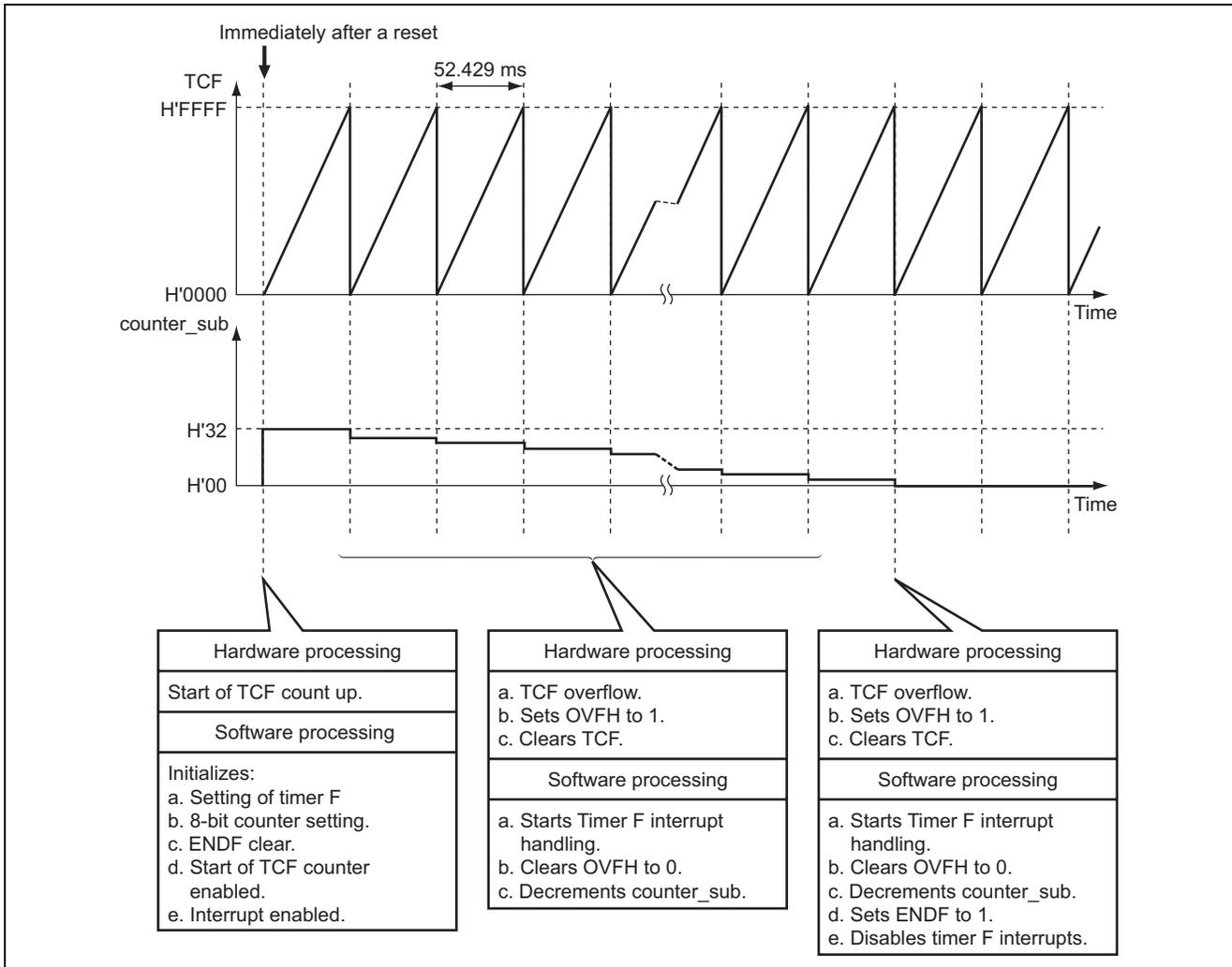
Figure 2 Operation Principle of Interrupt Counting by 16-Bit Timer Counter Function of Timer F
