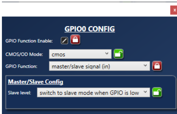
Figure 8. GPIO Configuration for Use with “GPIO_slave” Reference Mode
