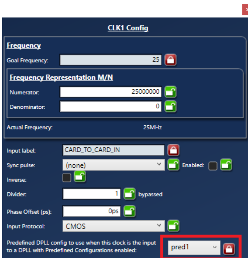
Figure 6. Card-to-Card Reference Configuration (clk1)
