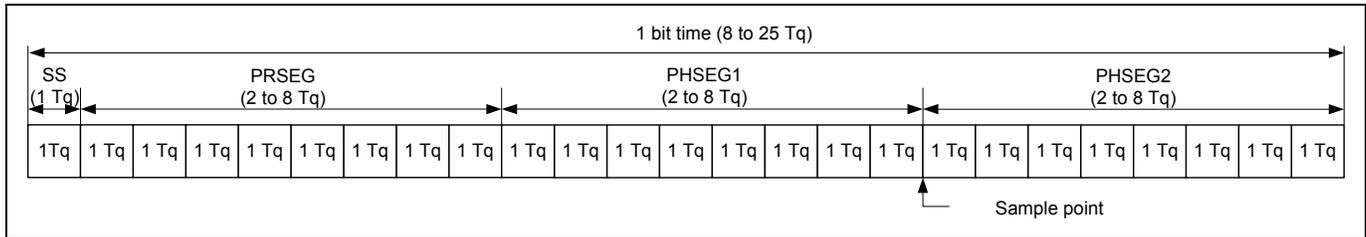
**Figure 4 Bit Configuration**
