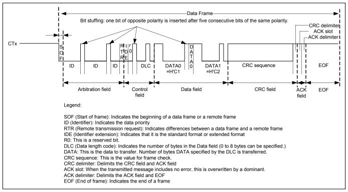
Figure 5 CAN Transmission Waveform
