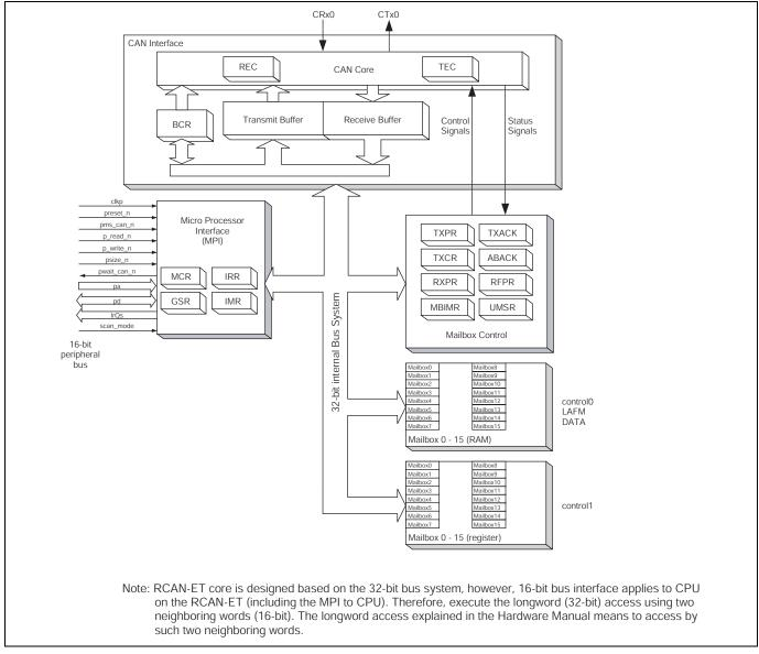
Figure 1 CAN Block Diagram
