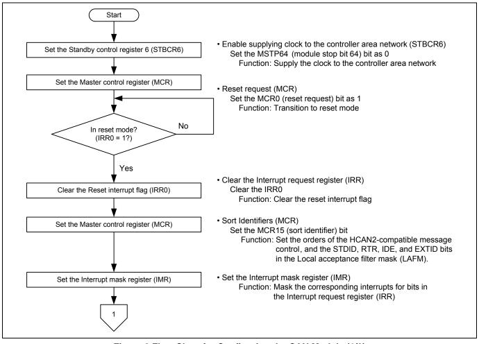
Figure 2 Flow Chart for Configuring the CAN Module (1/2)
