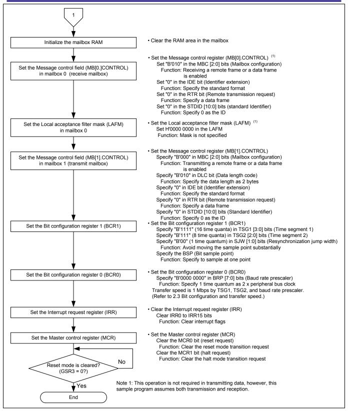
Figure 3 Flow Chart for Configuring the CAN Module (2/2)
