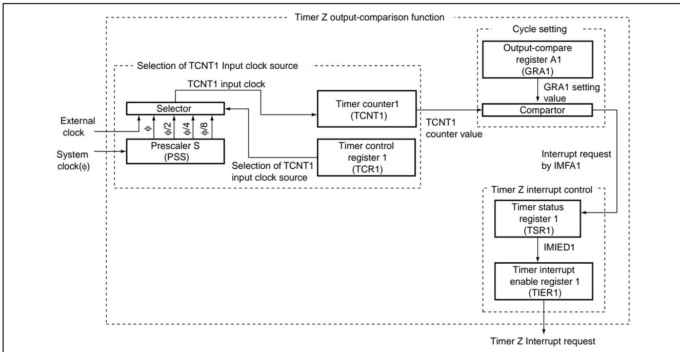
**Figure 3.3 Block Diagram of Interrupt Generation Per Magnetic-Field Switching Cycle by Timer Z's Output-Comparison Function**
