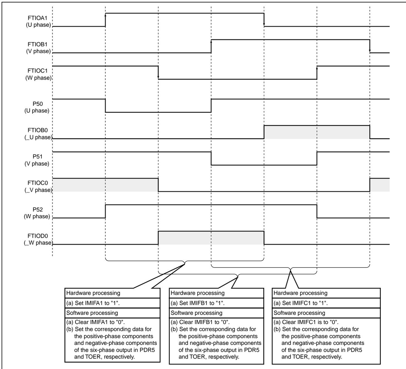
**Figure 4.2 Principle of Motor Control Based on the Rotor-Positional Signal**
