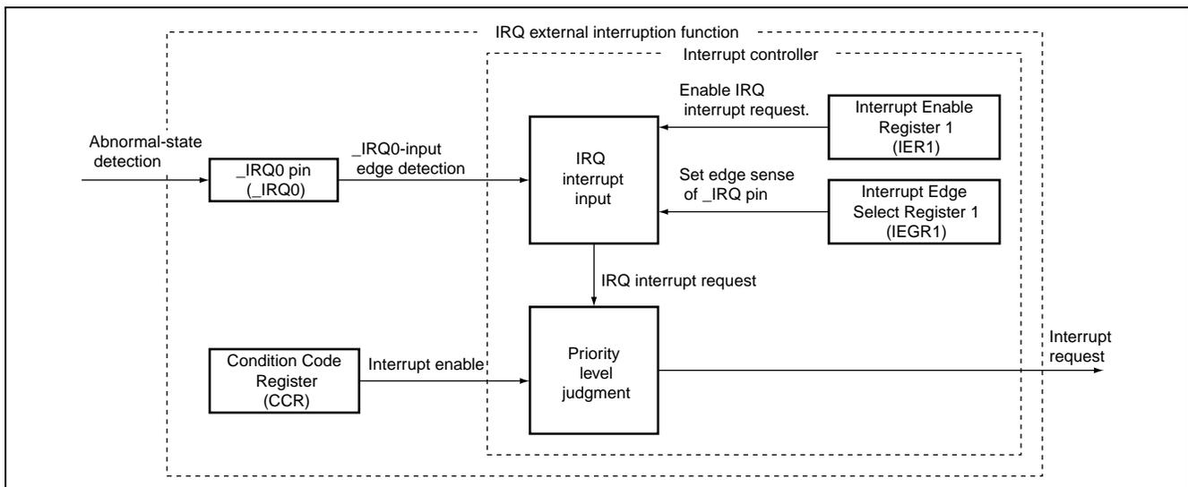
**Figure 3.6 Block Diagram of the Use of the IRQ External-Interrupt Function to Detect Abnormal States**
