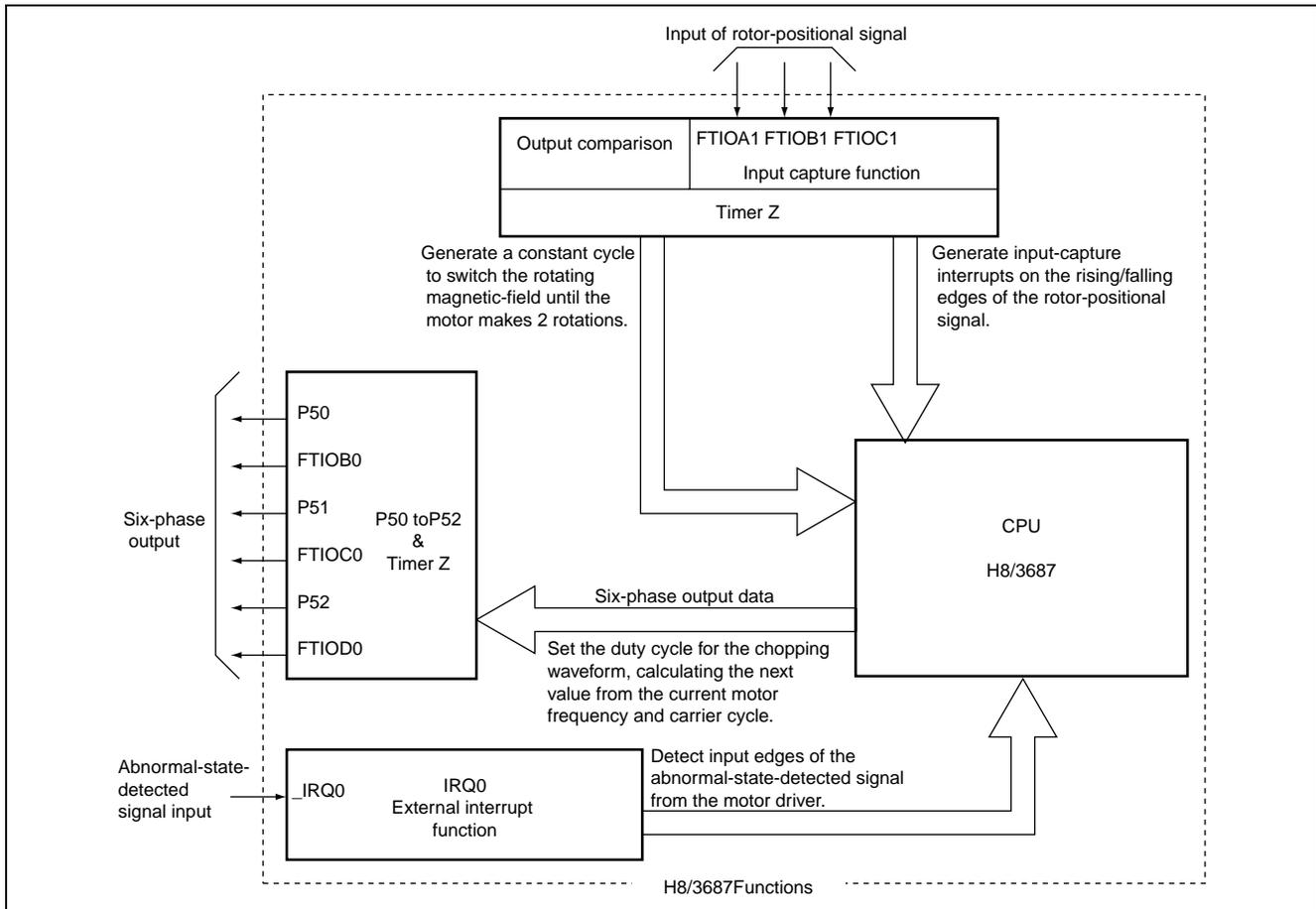
Figure 3.1 Block Diagram of the Configuration for Controlling a Brushless DC Motor
