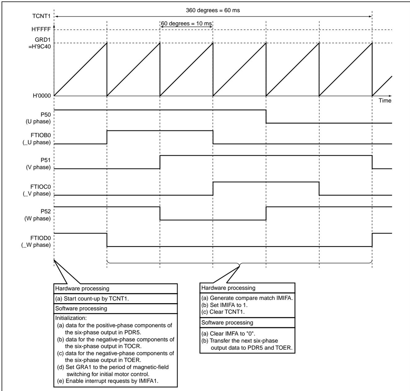
Figure 4.1 Initial Control of the Brushless DC Motor: Principle of Operation
