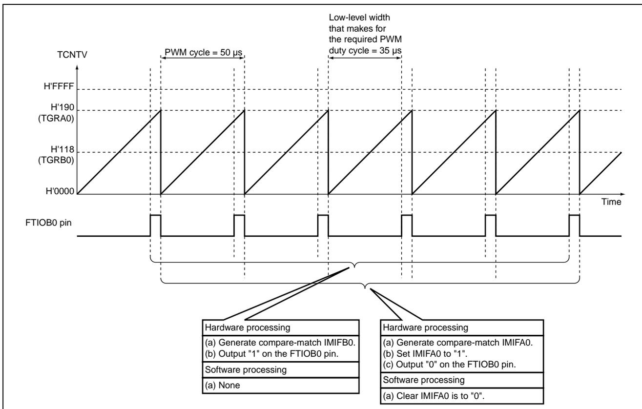
Figure 4.3 Output of the Chopping Waveform: Principle of Operation
