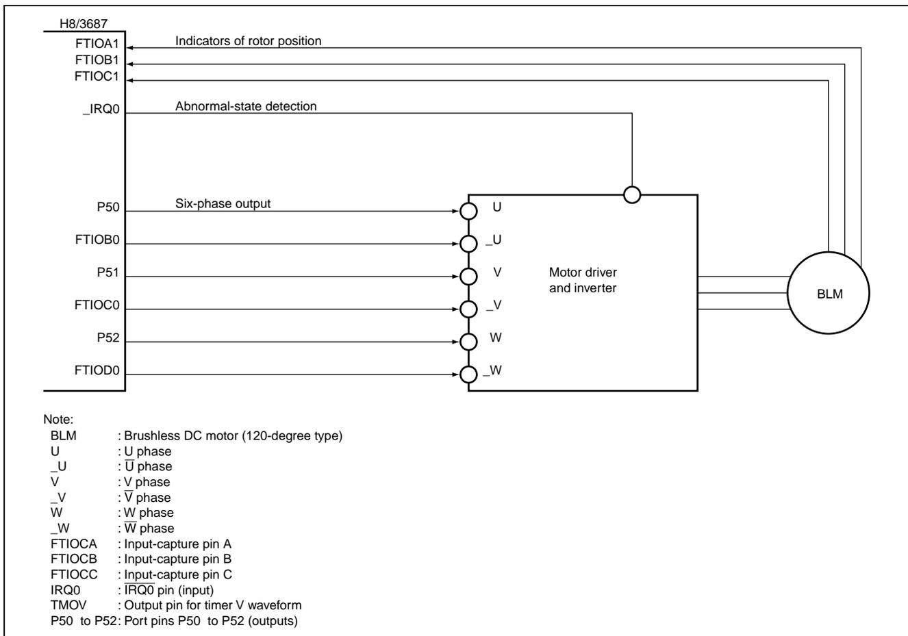
Figure 1.1 Set-up for Controlling a Brushless DC Motor
