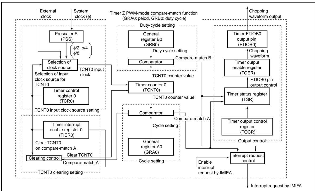
**Figure 3.4 Block Diagram of Chopping Waveform Output Using the PWM-Mode Compare-Match Function of Timer Z (CH0)**
