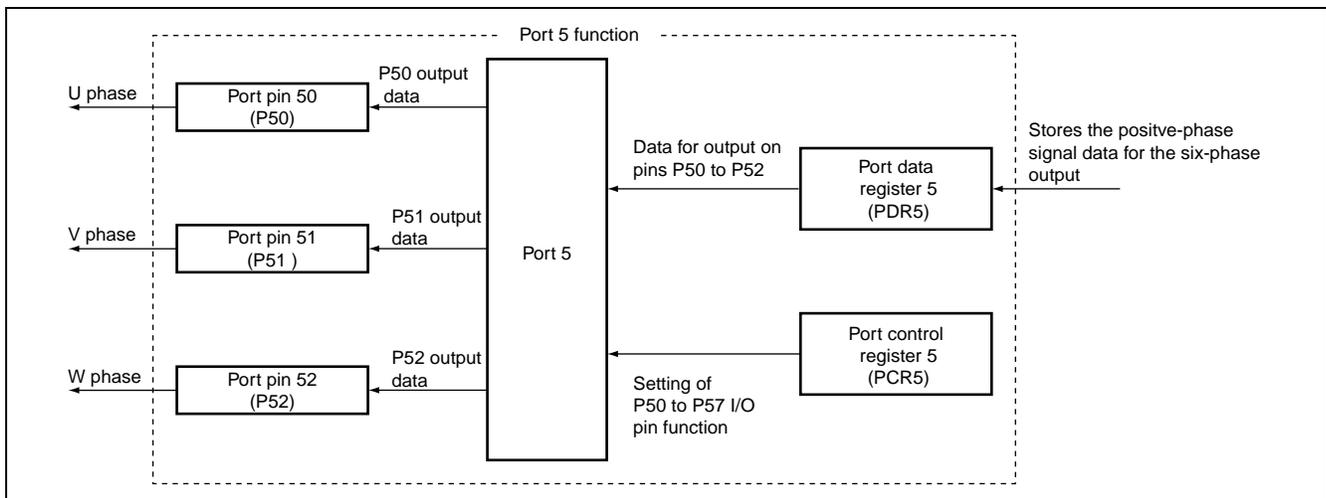
**Figure 3.5 Block Diagram of Six-Phase Output on Port 5**
