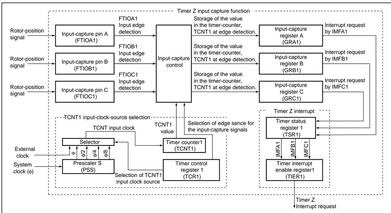
**Figure 3.2 Block Diagram of Interrupt Generation by the Input-Capture Function in Response to Edges of the Rotor-Positional Signal**
