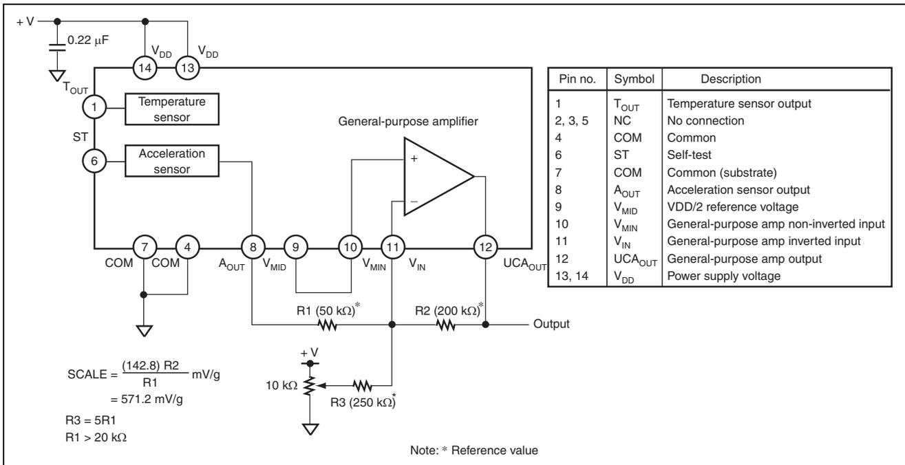
**Figure 1.2 Application Circuit with Increased Scale Factor (Reference)**
