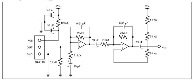
Figure 1.2 Example of Sensor Output Amplifier Circuit (Reference)
