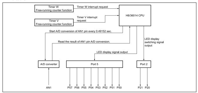
Figure 2.1 Block Diagram of the Functions in Use
