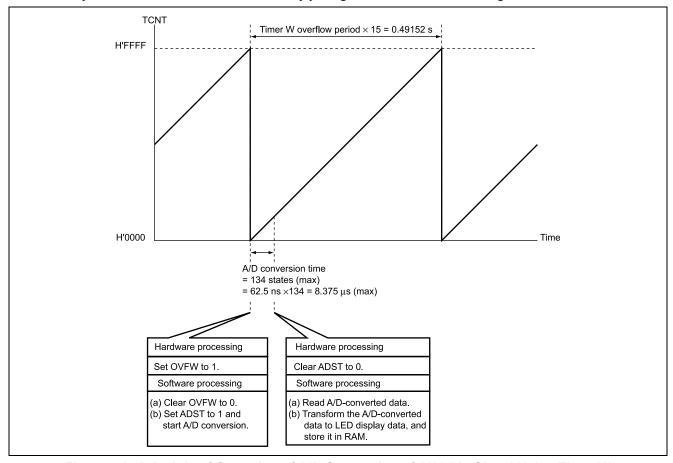
Figure 3.1 Principle of Operation of A/D Conversion of AN1-Pin Signal Using Timer W
