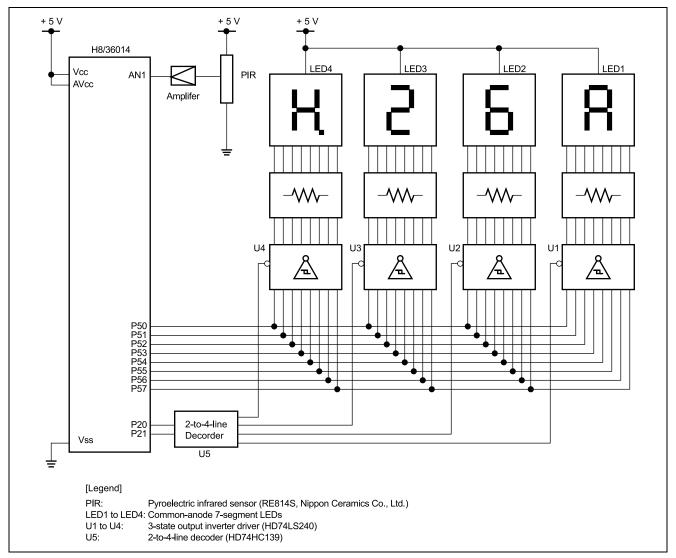
Figure 1.1 Hardware Configuration
