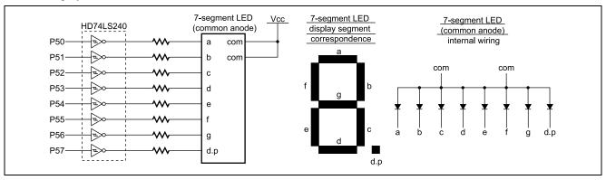
Figure 2.2 7-Segment LED Connections and Internal Wiring
