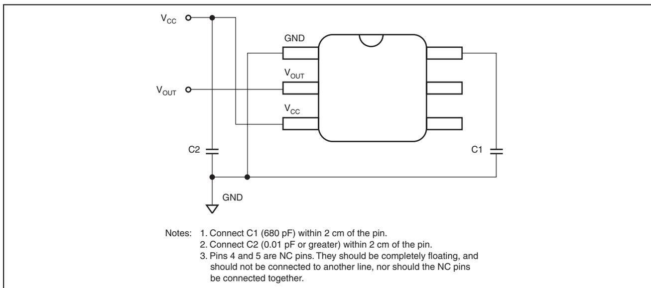
**Figure 1.2 Connection Diagram (Reference)**
