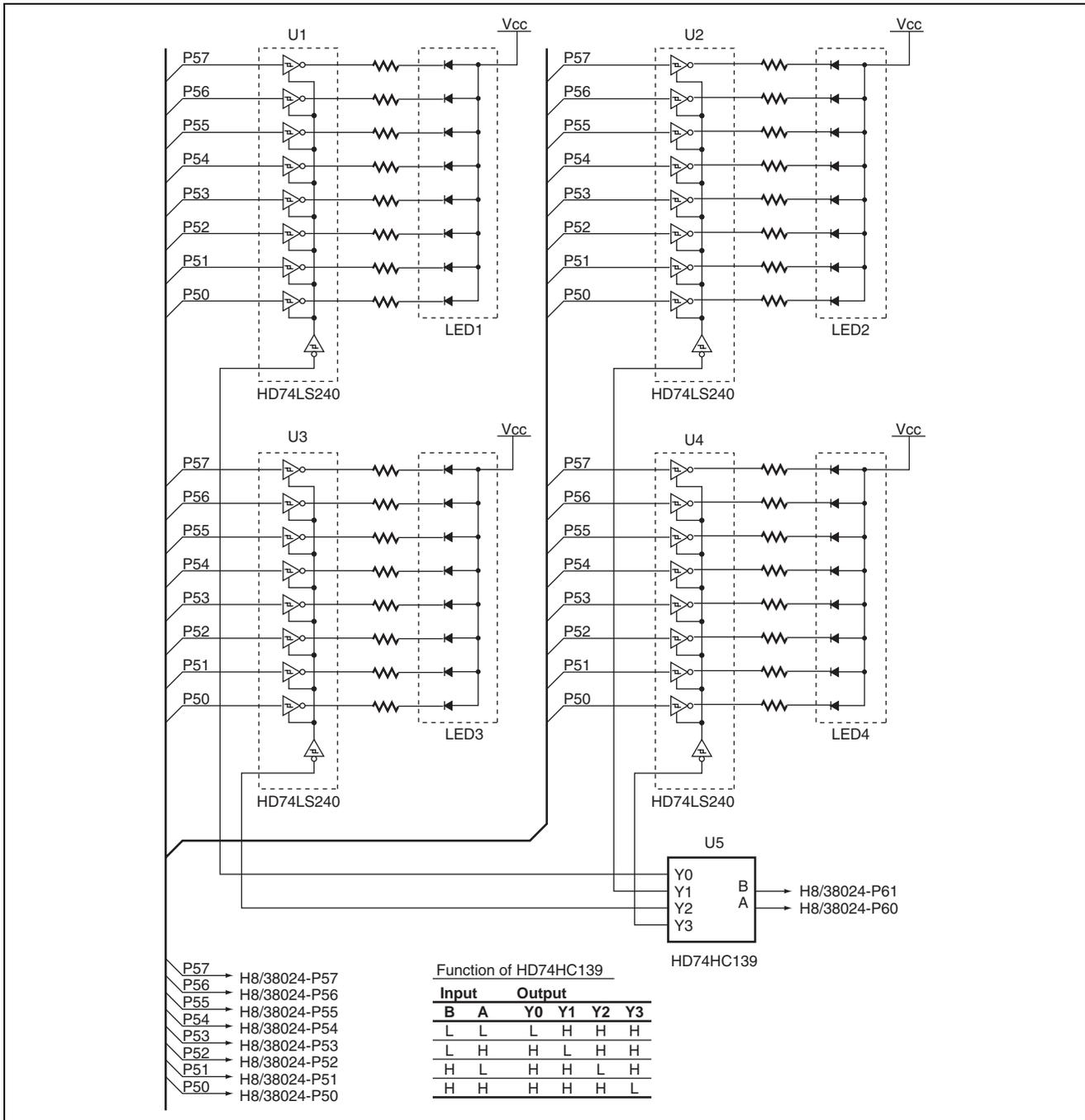
**Figure 1.4 Control of 7-Segment LEDs**
