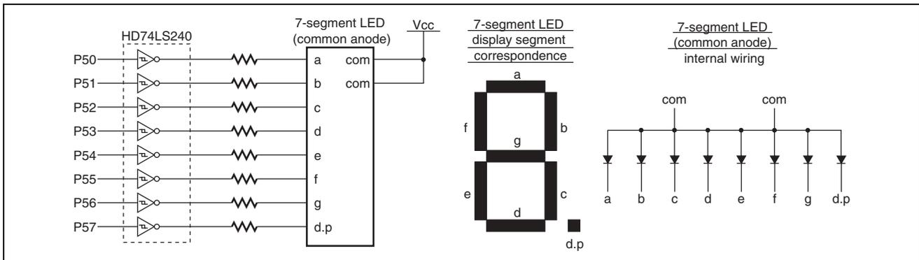
**Figure 2.2 7-Segment LED Connection and Internal Wiring**
