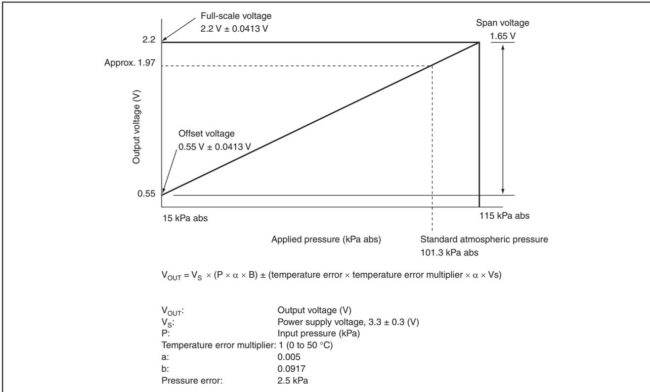
**Figure 1.3 Output Characteristics (Reference)**
