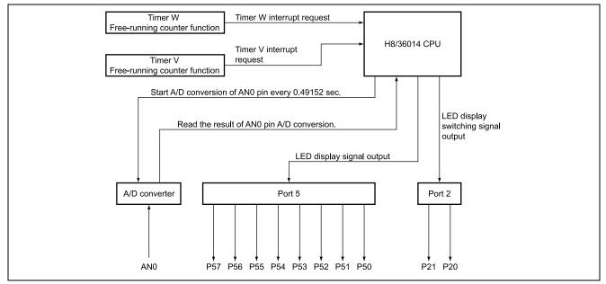
Figure 2.1 Block Diagram of Functions
