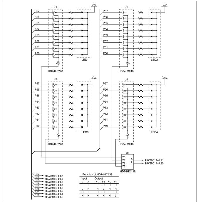
Figure 1.4 Control of Seven-Segment LEDs
