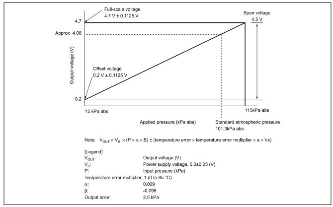
Figure 1.3 Output Characteristics (Reference)
