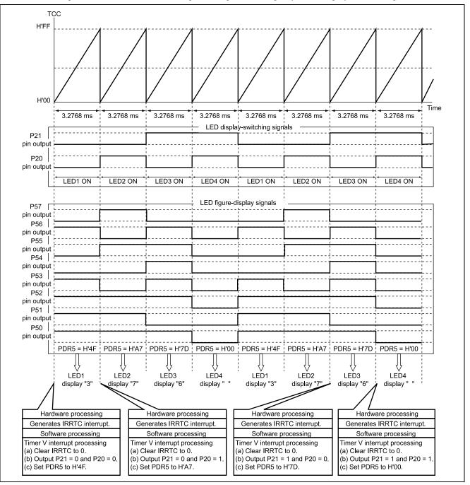
Figure 3.2 Principle of Operation for the 7-Segment LED Display Control
