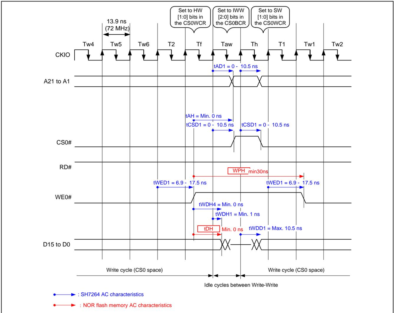
Figure 8 Write Timing Example When Using Random Access Read (2)
