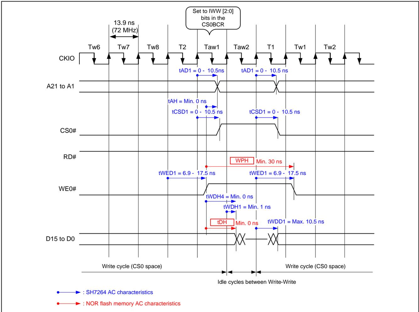
Figure 12 Write Timing Example When Using Page Read (2)
