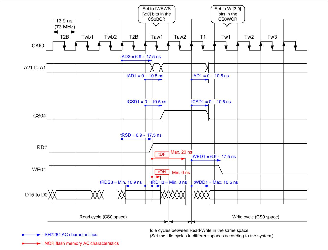
Figure 10 Read Timing Example When Using Page Read (2)
