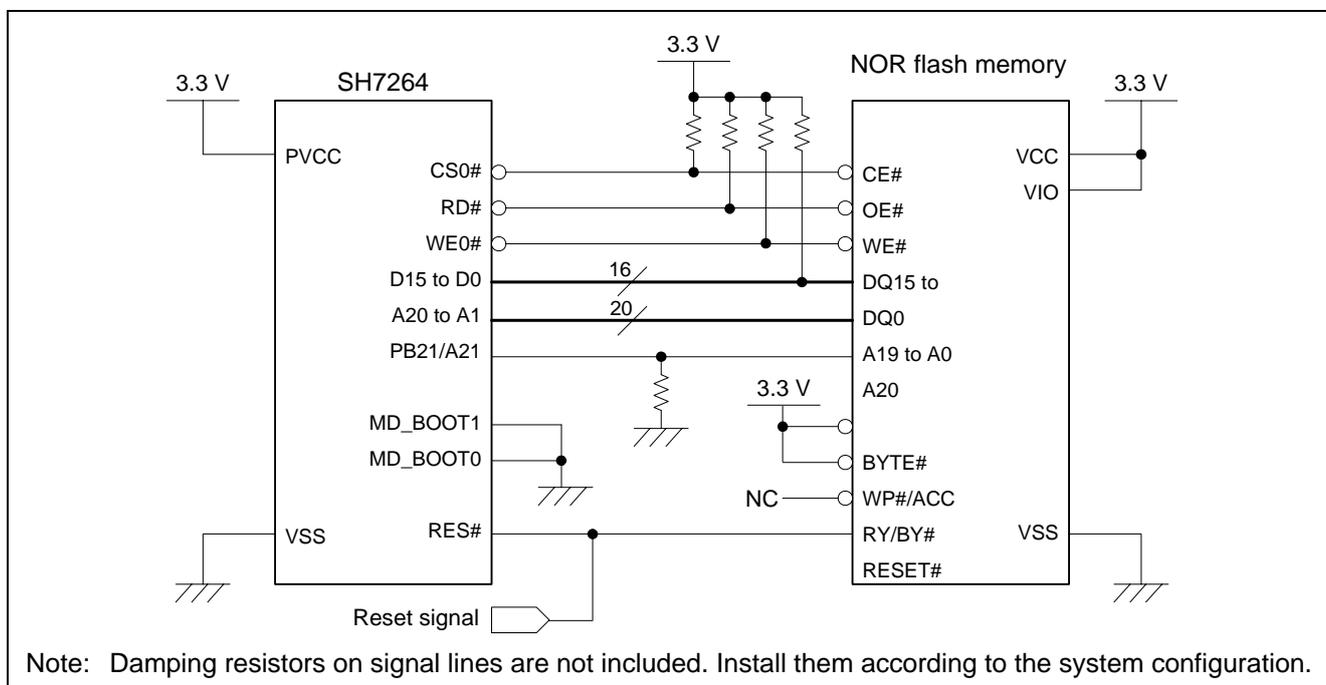
**Figure 2 NOR Connection Circuit**
