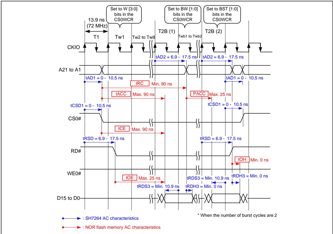
Figure 9 Read Timing Example When Using Page Read (1)
