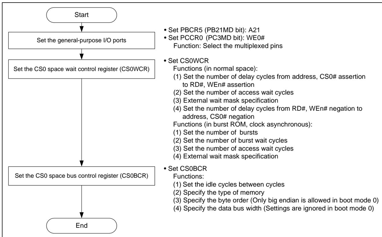
**Figure 4 Bus State Controller and General-purpose I/O Port Setting Procedure (CS0 Space)**
