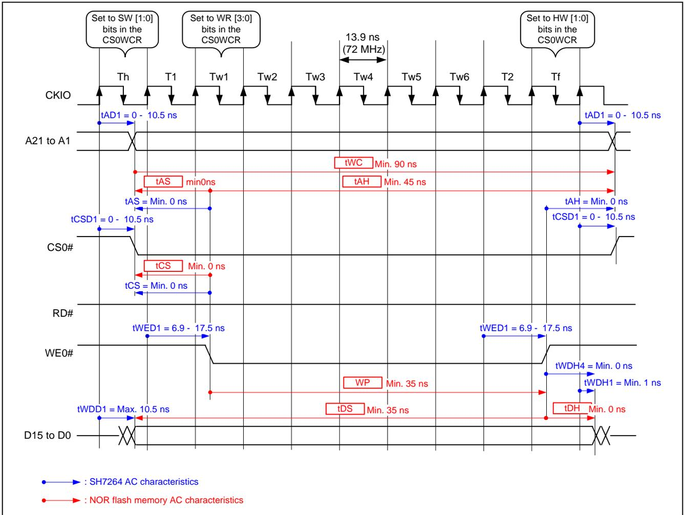
Figure 7 Write Timing Example When Using Random Access Read (1)
