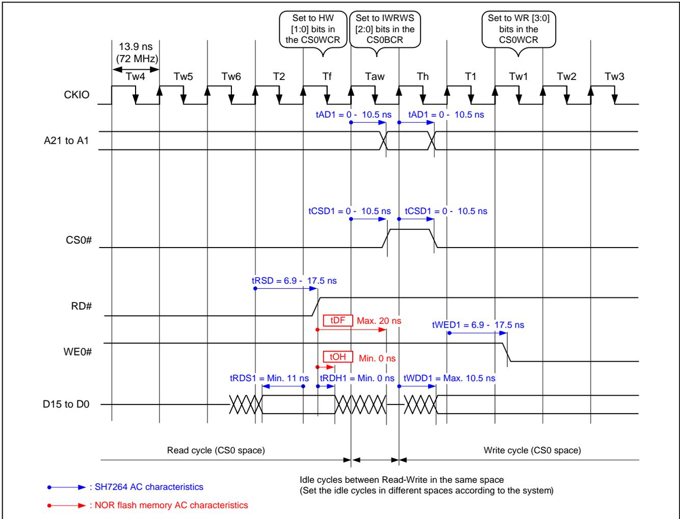
Figure 6 Read Timing Example When Using Random Access Read (2)
