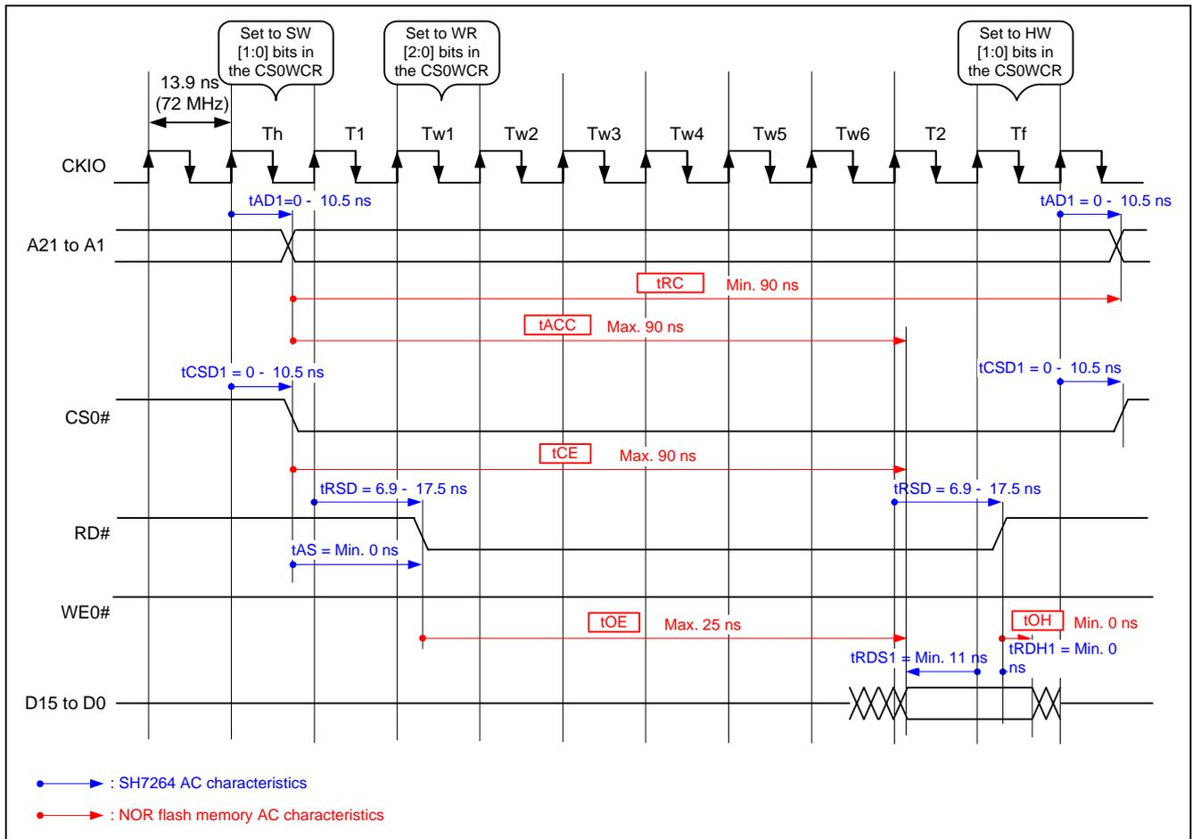
Figure 5 Read Timing Example When Using Random Access Read (1)
