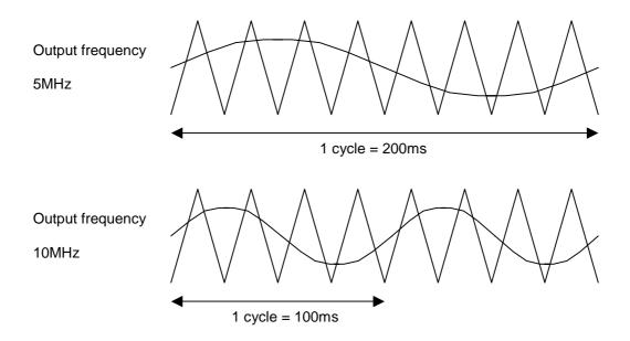
Figure 5.10 Altering the Output Frequency
