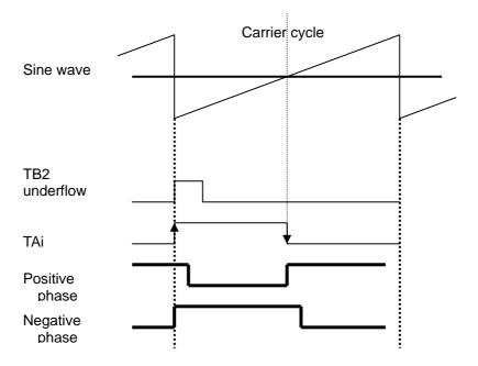
Figure 4.2 Relationship between Timer and PWM during Sawtooth Wave Modulation
