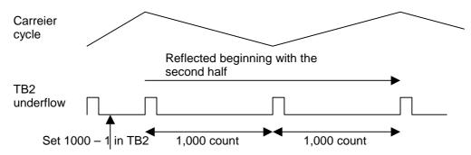
When TB2 is reloaded at odd-numbered occurrences of timer A output (tb2sc = 00000001B)
