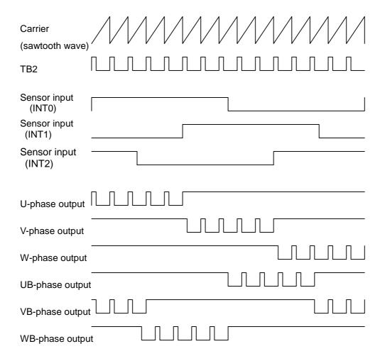
Figure 6.1 Relationship between 120-degree Turn-on Control Sensor Input and Waveform Output
