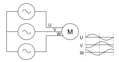
Figure 3.1 Three-phase Motor Drive
