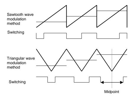
Figure 4.1 Carrier Frequency Modulation Method
