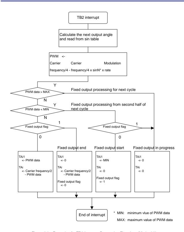
Figure 5.9 Example of a TB2 Interrupt Processing Flowchart (Method 2)
