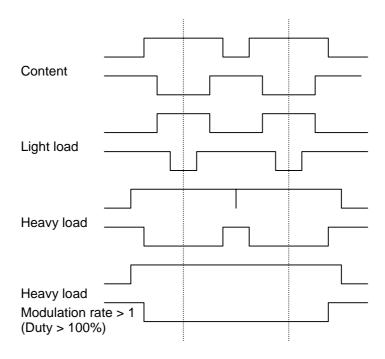
Figure 5.4 Relationship between Modulation Rate and Output Waveform
