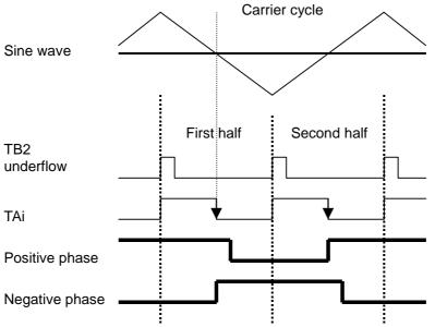
The first half and the second half basically are considered to be symmetrical. (Actually, inclined and not symmetrical because they are arced parts of a sine wave.)
