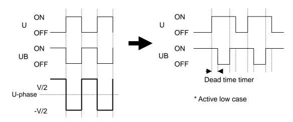
Figure 3.4 Microcomputer Output Waveform and Generated Waveform
