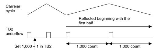
Figure 4.10 Carrier Cycle Settings and Refection
