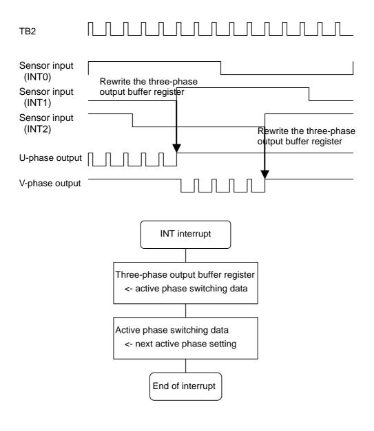
Figure 6.2 Sensor Interrupt and Output Phases
