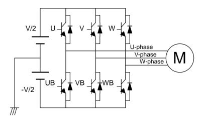
Figure 3.3 Power Transistor Circuit
