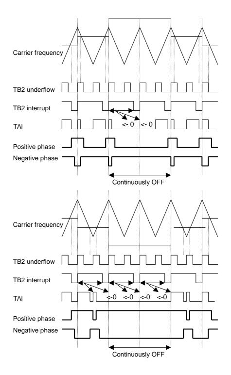
Figure 5.8 Relationship between TAi Data Setup Timing and Reflection
