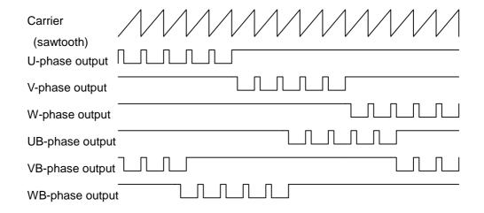
Figure 4.12 Conceptual Waveform of 120-degree Turn-on Output (see Section 6 for details)
