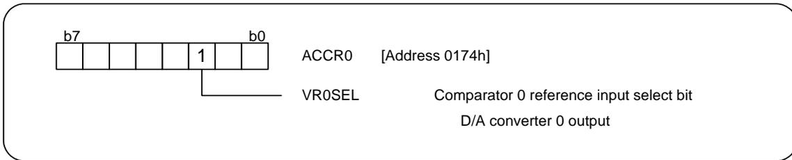
(7) Set the D/A0 output to enable.
