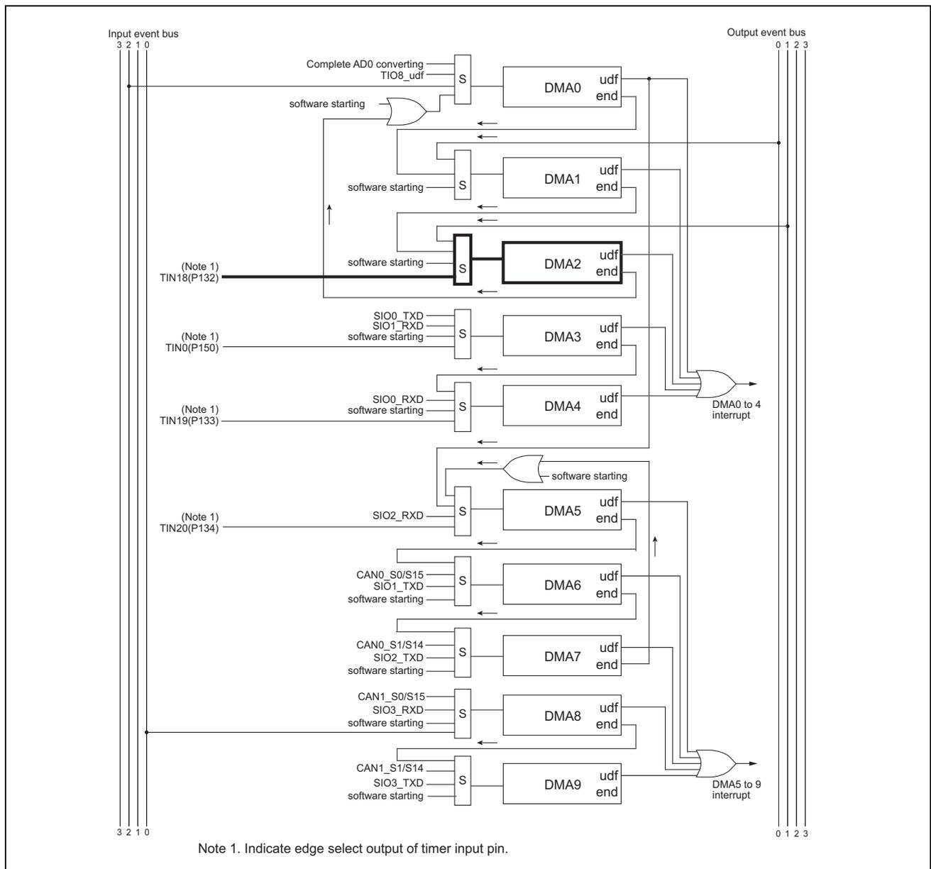
Figure3.1.1 Configuration of Sample for Combination of input pin and DMAC
