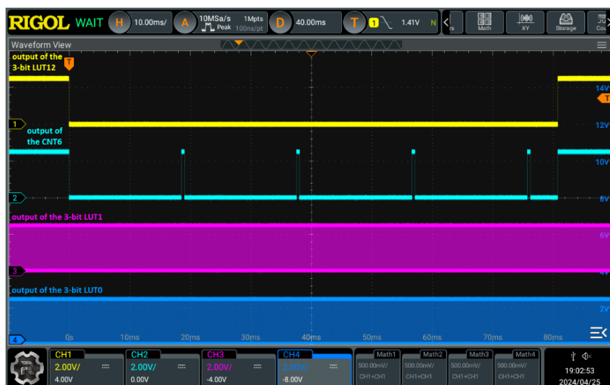
Figure 5: The duration of the low signal level from 3-bit LUT12 (yellow upper line) indicating the unlocking of the CNT6 counter (teal) corresponds to the duration of pressing the SB1 or SB2 buttons
