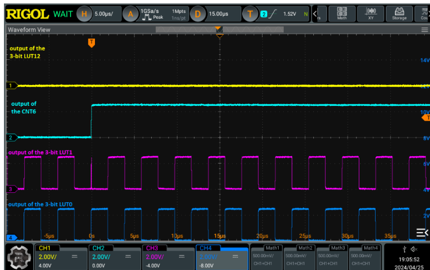
Figure 7: Zoomed-in image of Figure 5. The polarity of the clock frequency of the corresponding multiplexers corresponds to the decreasing value of the duty cycle (when the SB1 button is pressed)
