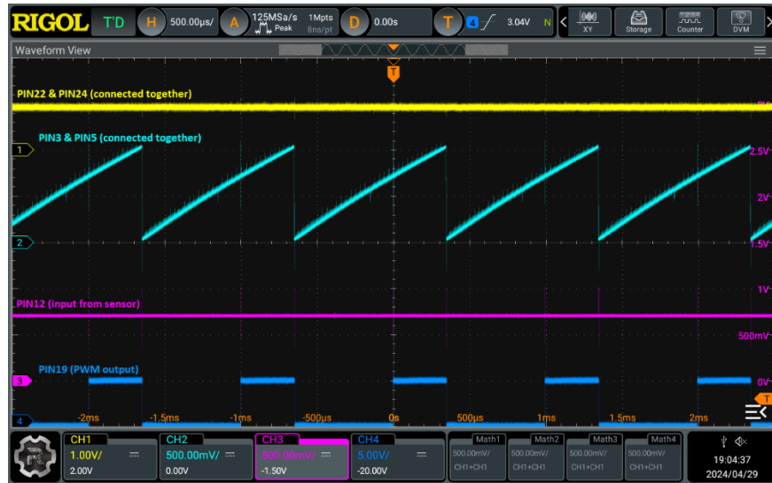
Figure 16: Operation of the PWM generation circuit. Duty cycle is ~35%
