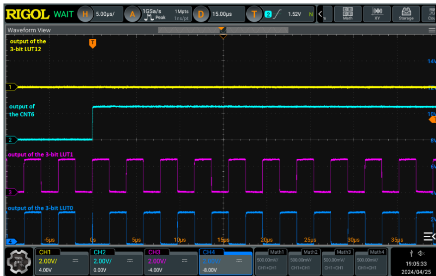
Figure 6: Zoomed-in image of Figure 5. The polarity of the clock frequency of the corresponding multiplexers corresponds to the increasing value of the duty cycle (when the SB2 button is pressed)
