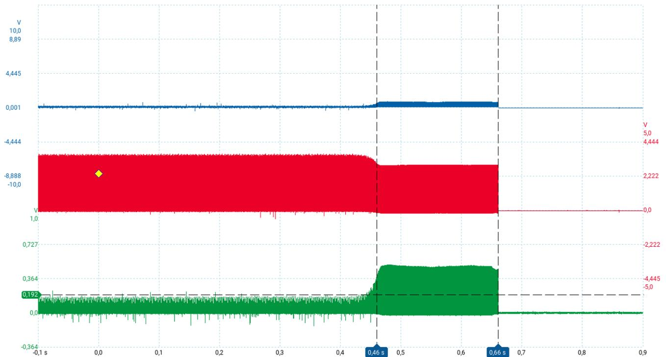
Figure 11. Hold-to-Stop Operation, Whole Trace
