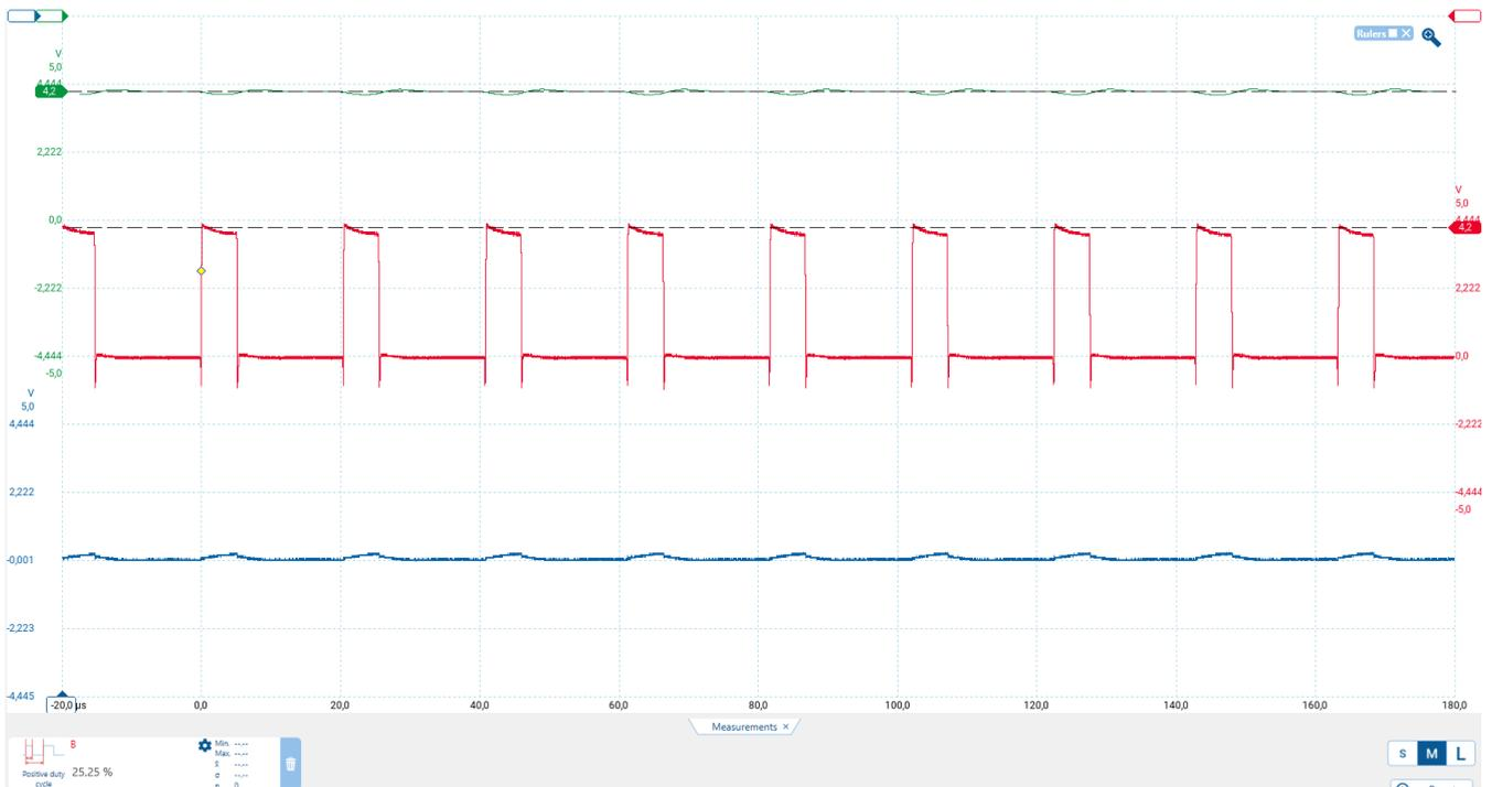
Figure 7.  $V_{DD} = 4.2\text{ V}$ , duty cycle 25.25%
