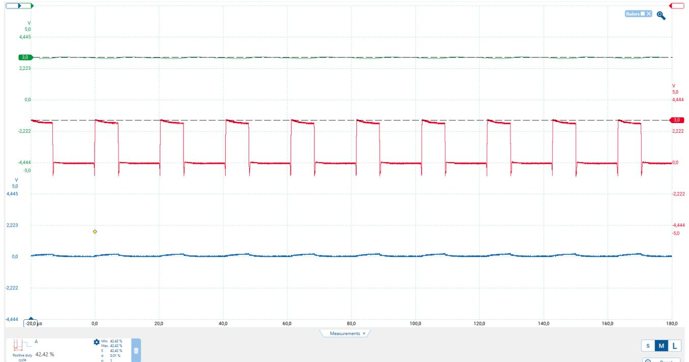
Figure 5.  $V_{DD} = 3.0\text{ V}$ , duty cycle 42.42%
