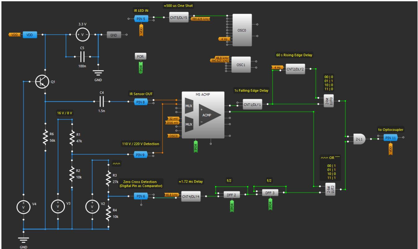
Figure 2. Automatic Hand Dryer GreenPAK Designer Schematic
