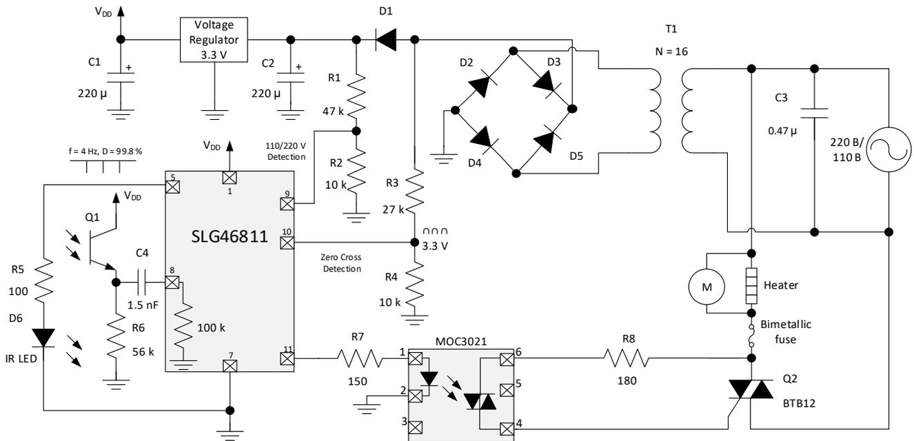
Figure 1. General Schematic of Automatic Hand Dryer Based on SLG46811
