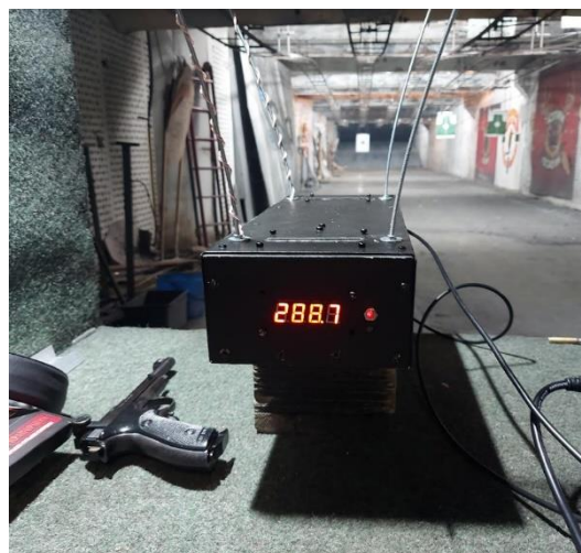
Figure 27: Cartridge Federal American Eagle CP Solid cal. 22 LR 45 gr. Beginning speed 295 m/s. Shot from Margolin pistol
