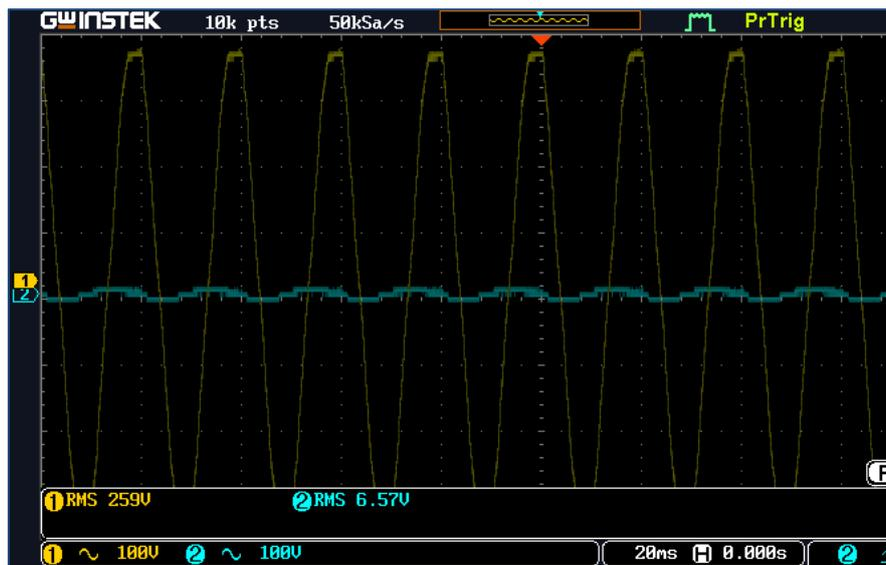
Figure 11: Overvoltage Condition
