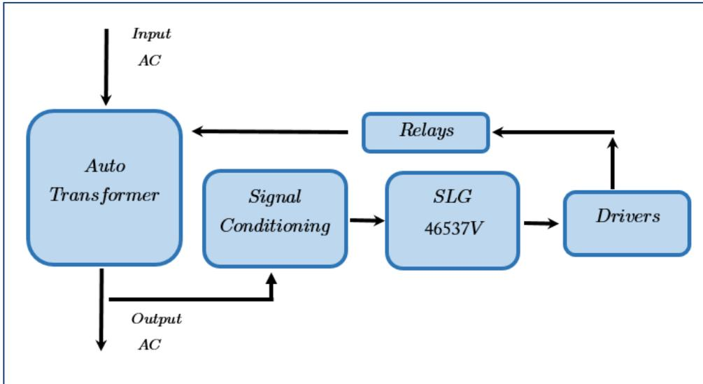
**Figure 1: Block Diagram**
