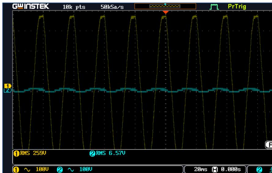
Figure 11: Overvoltage Condition
