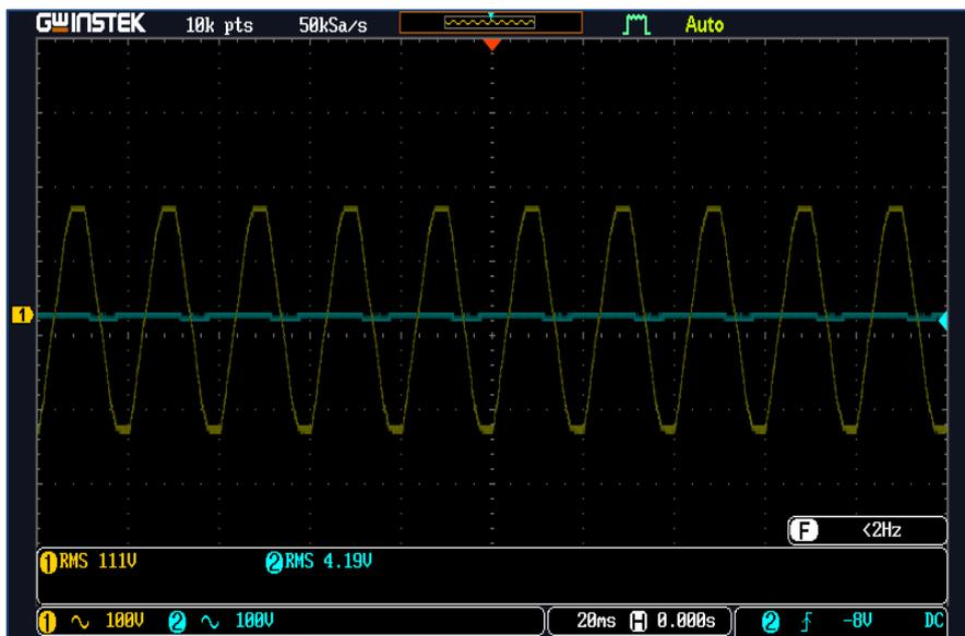
**Figure 13: Undervoltage Condition**
