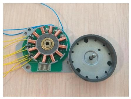
**Figure 1: BLDC Motor Construction**
