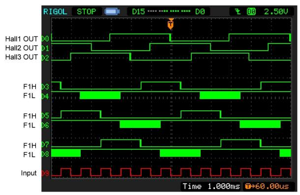
Figure 6: BLDC Motor Operation Scope Shot
