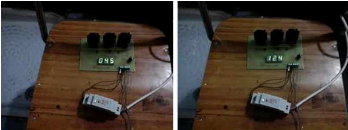
Figure 9: Tests with Water Flow Sensor and Home Water Source at Two Different Flow Rates
