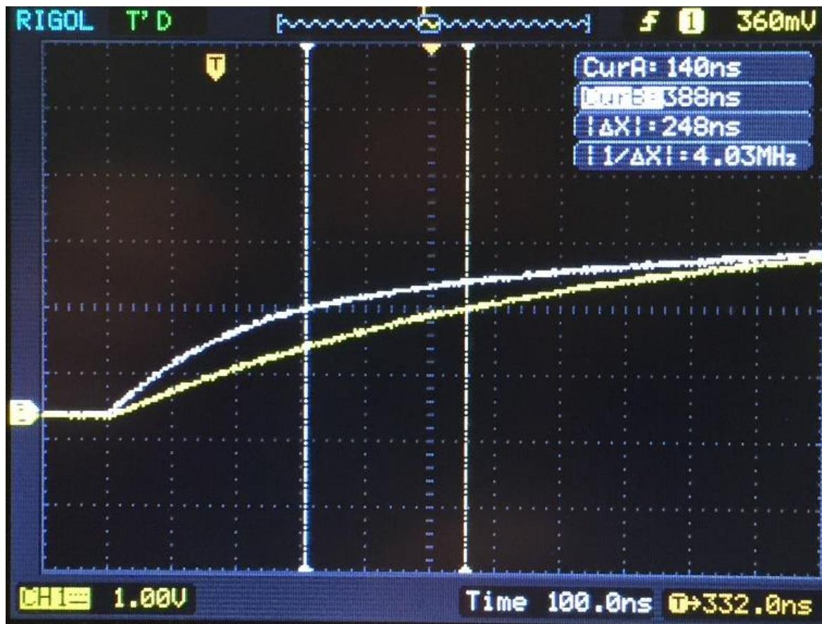
Figure 2: Oscilloscope Capture Showing the Difference in Risetime
