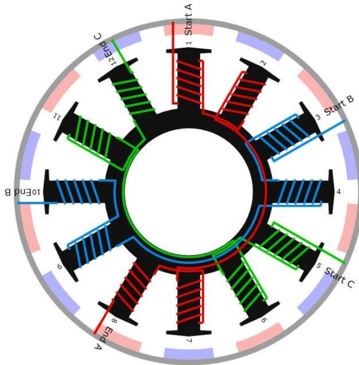
Figure 2: BLDC Motor Coil Placement
