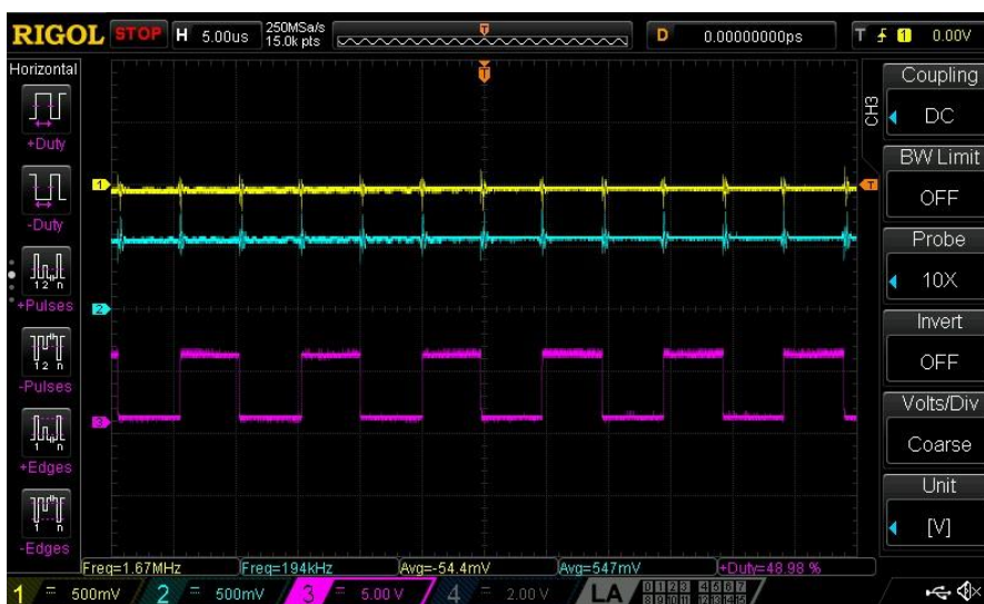
Figure 12: 50% Output Duty Cycle, ANALOG_IN \approx 550 mV
