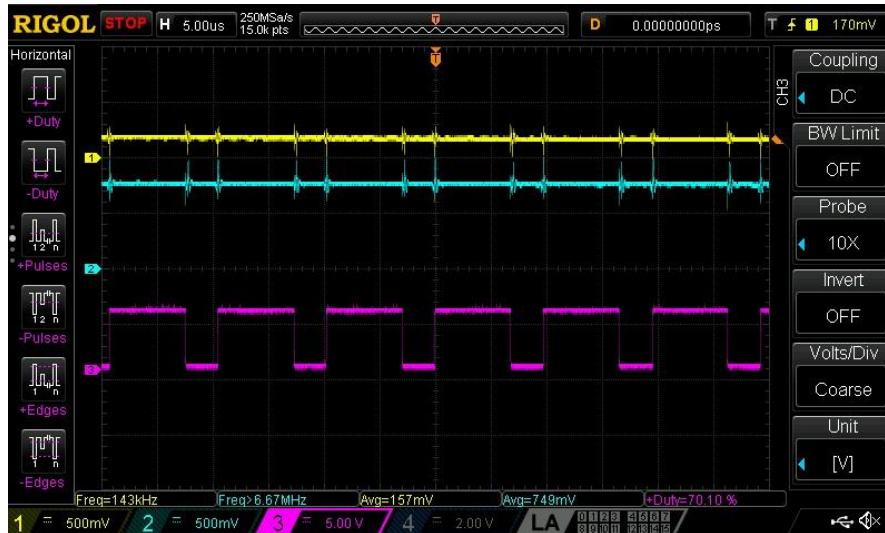
Figure 11: 70% Output Duty Cycle, ANALOG_IN \approx 700 mV
