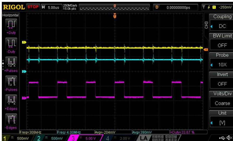
Figure 13: 30% Output Duty Cycle, ANALOG_IN \approx 400 mV
