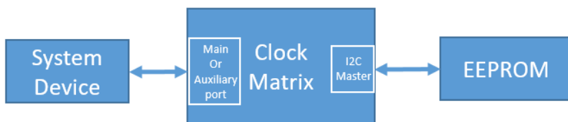
Figure 3. Programming the EEPROM through Clock Matrix
