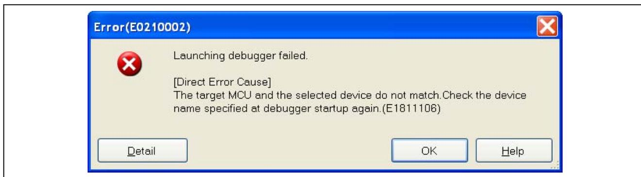
Figure 1.11 The Target MCU and the Selected Device Do Not Match
