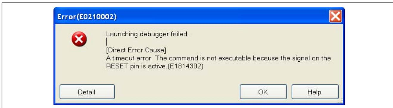
Figure 1.15 The Signal on the RESET Pin is Active
