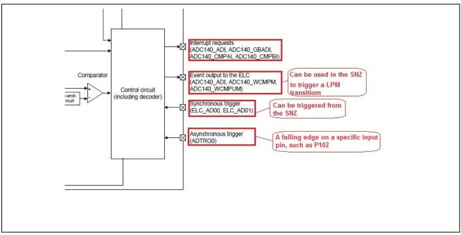
Figure 8. Input and output events for ADC14
