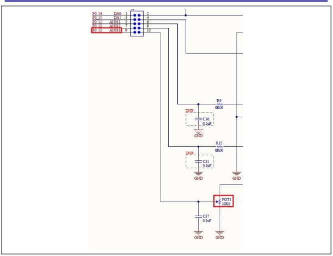
Figure 7. Potentiometer connection to the analog channel 13 on DK-S3A7
