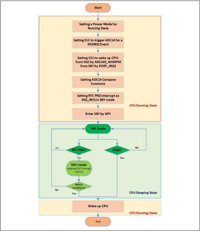
Figure 9. Algorithm used for checking ADC conditions in the Snooze mode
