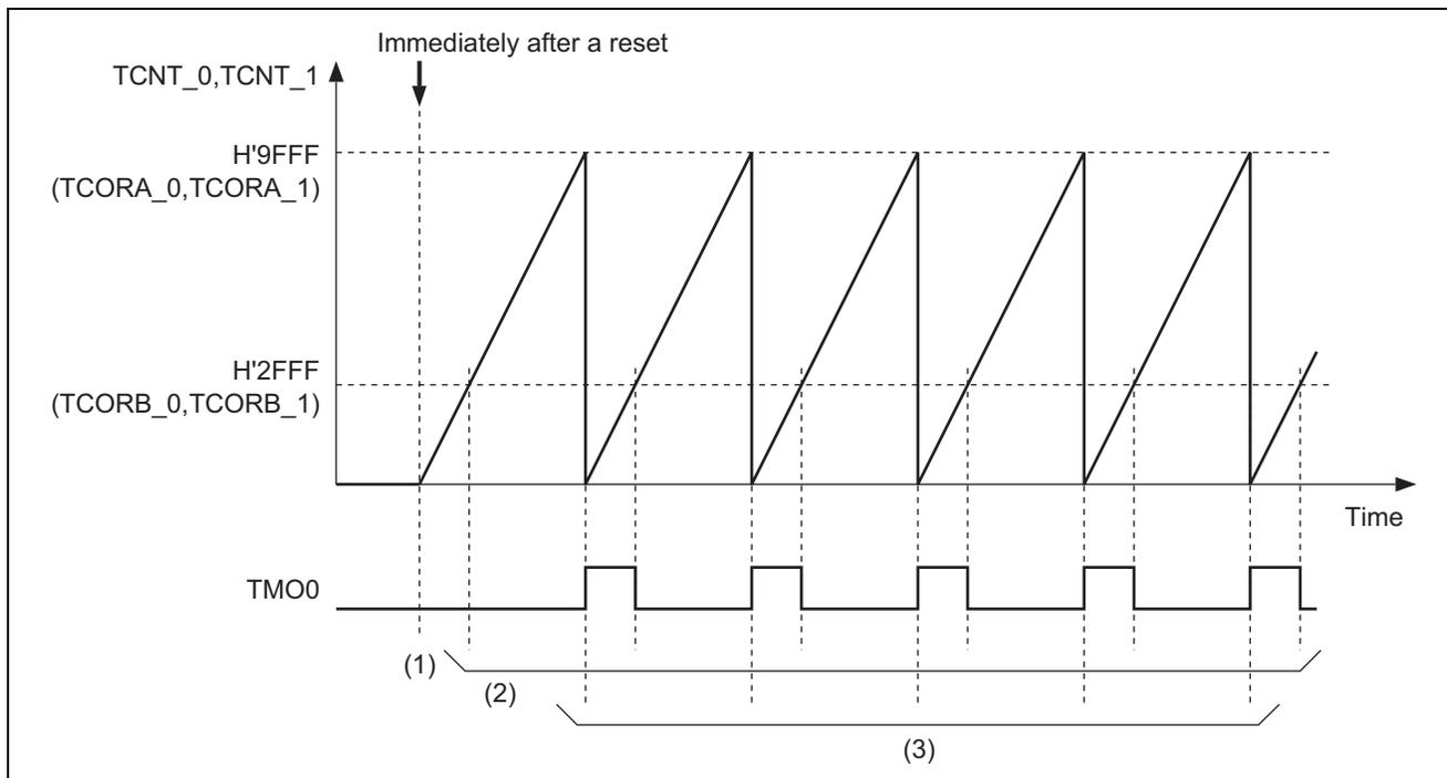
**Figure 3 Illustration of the Operation of Cascade-Connected 8-Bit Timers**
