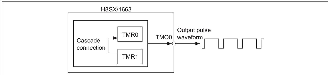
Figure 1 Example of Pulse Output by Cascade-Connected 8-Bit Timers
