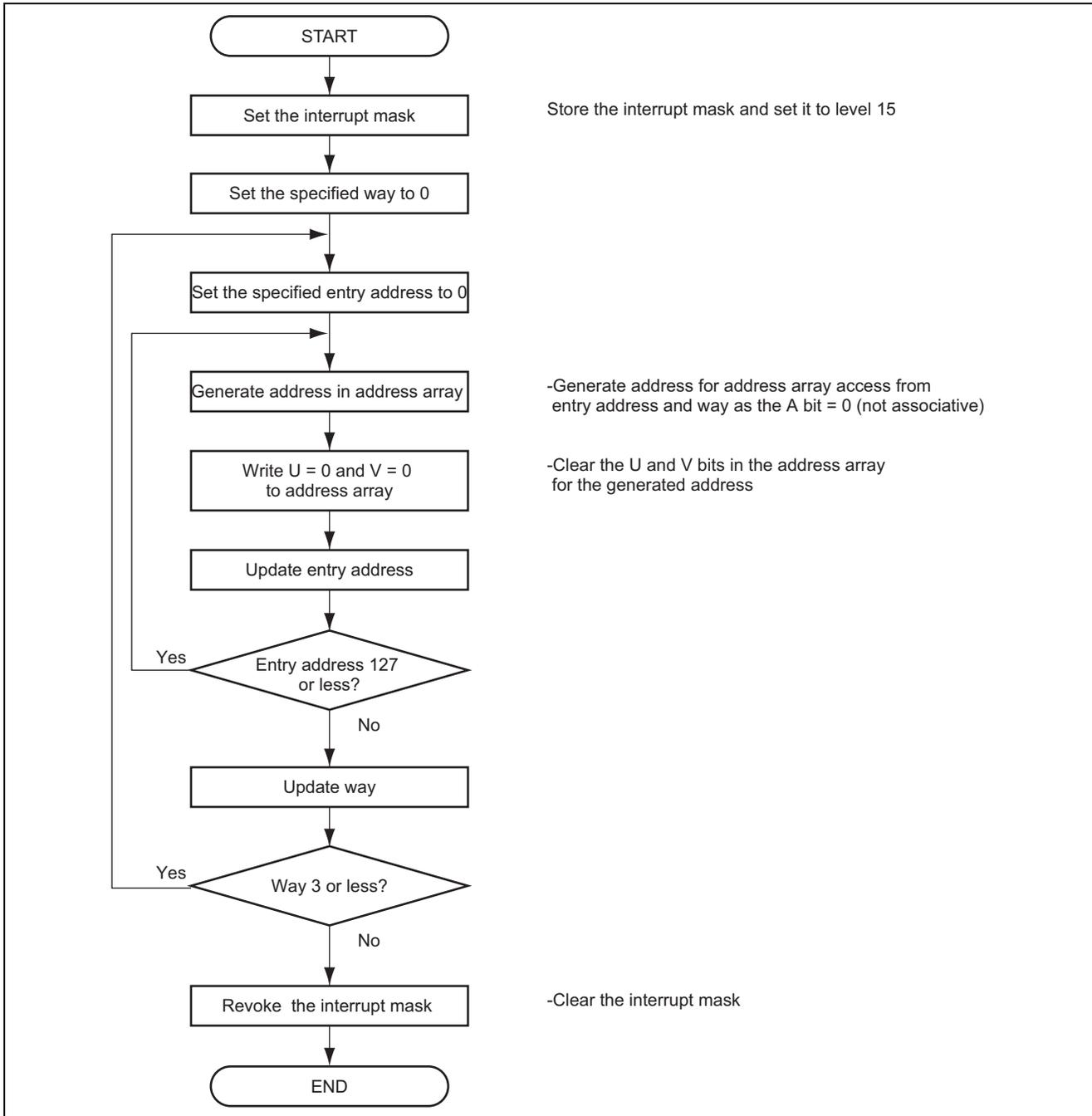
Figure 3 Example of Processing Flowchart for the Operand Cache Write-Back
