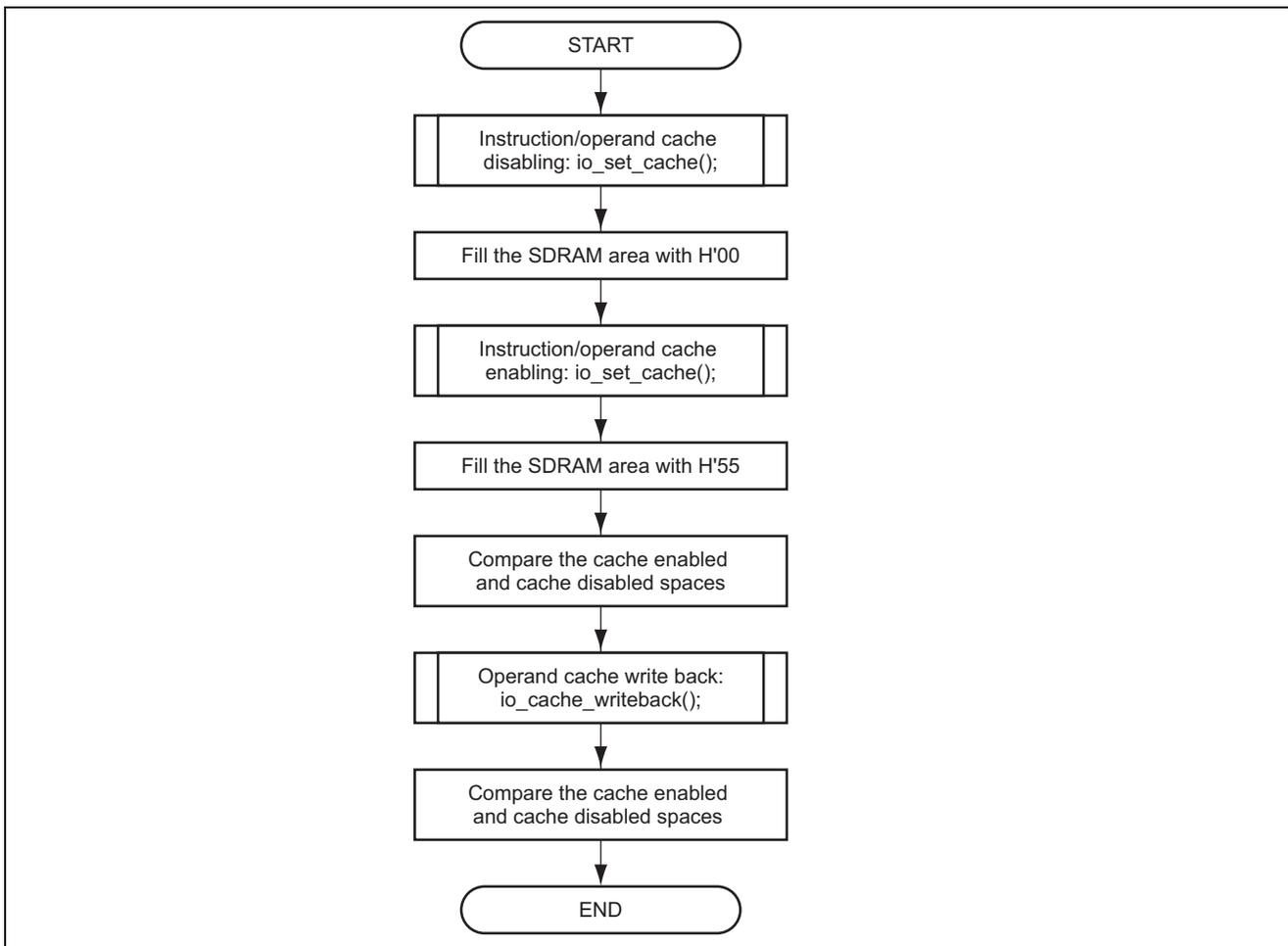
Figure 4 Flow of Processing by the Sample Program
