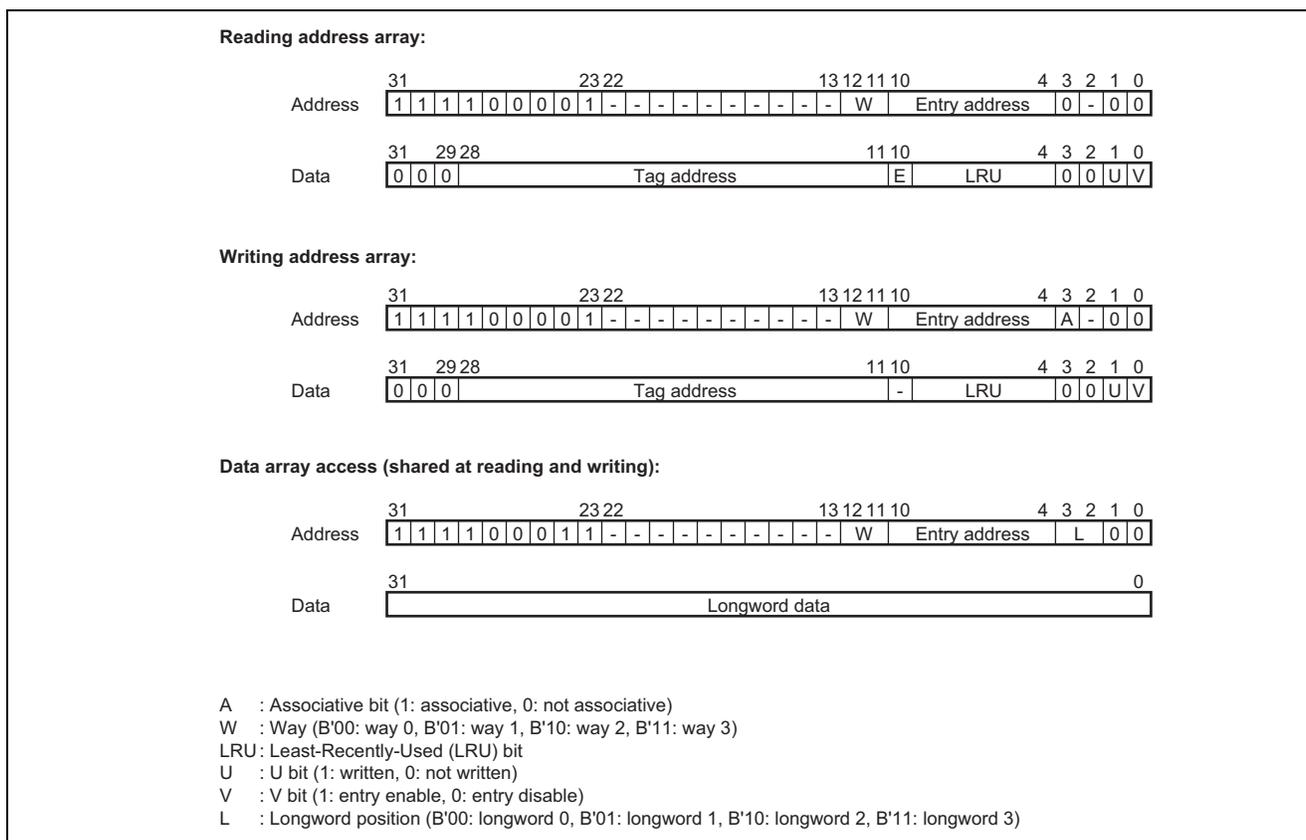
**Figure 2 Cache Access Specifying Method for Memory Allocation (Operand Cache)**
