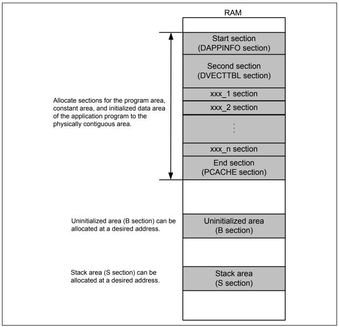
Figure 8 Application Program Section Alignment
