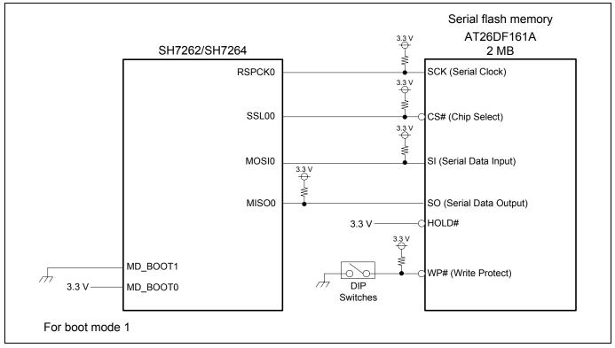
Figure 4 Connection Circuit for the SH7264 and Serial Flash Memory
