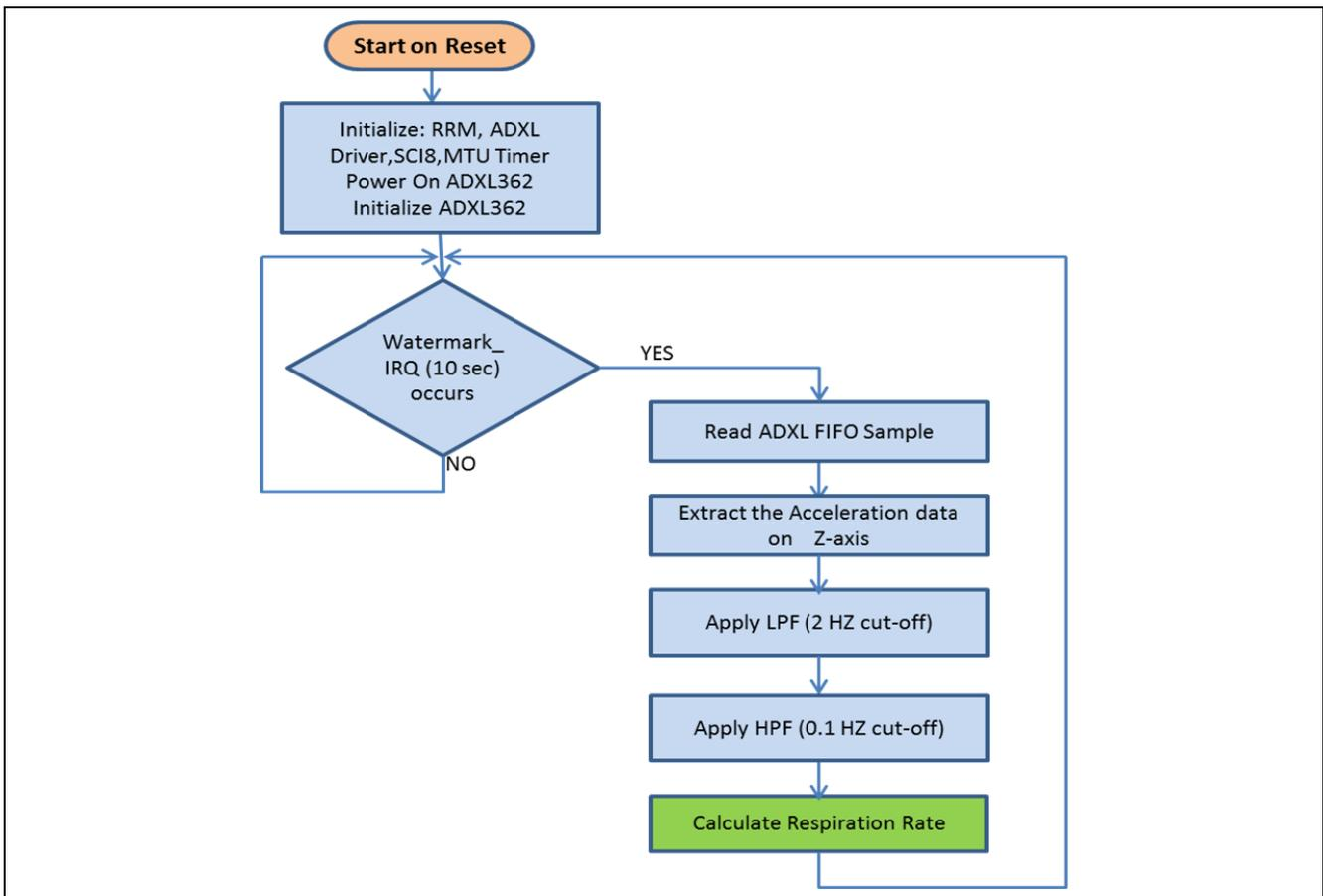
Figure 5-4 RRM Software Control Flow
