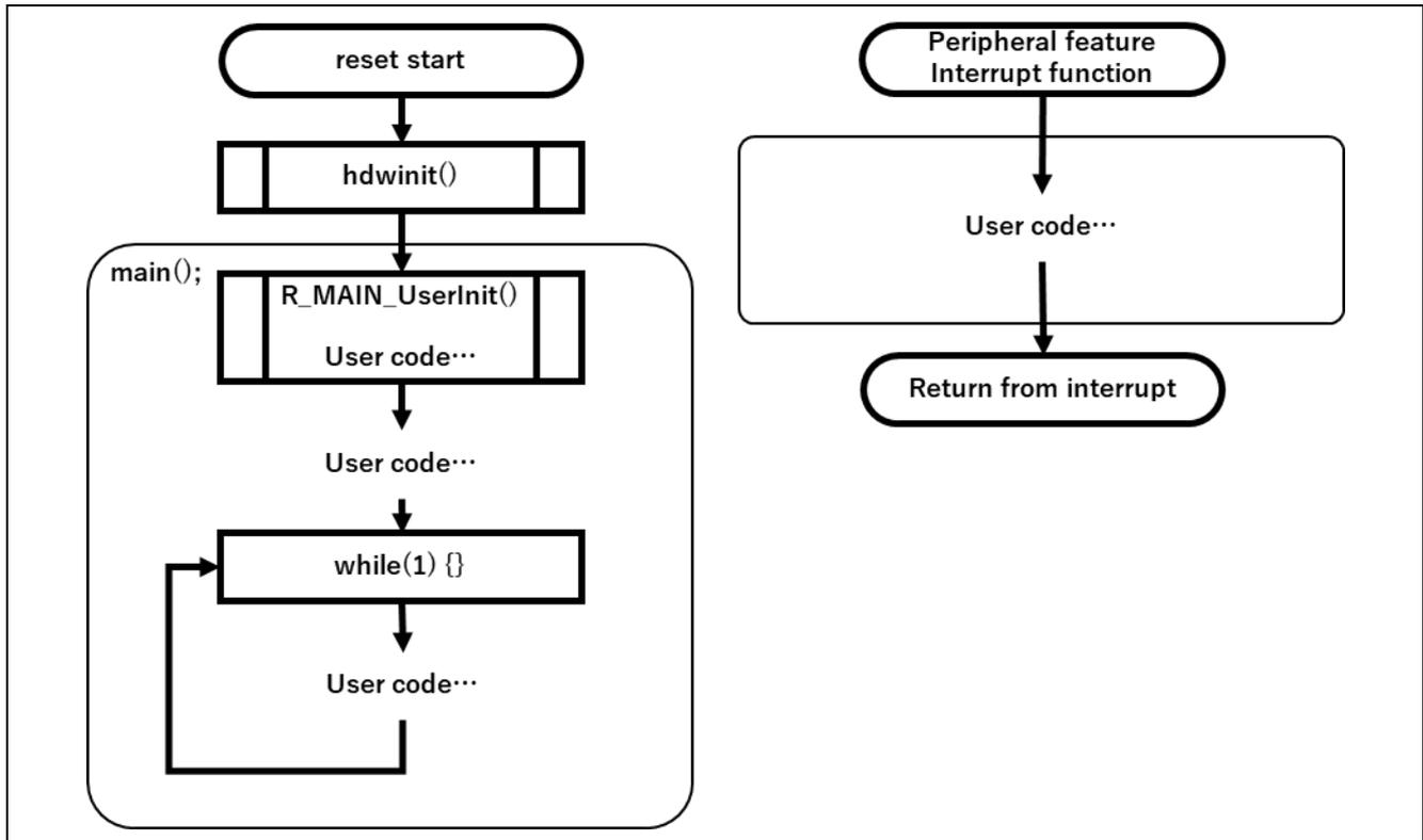
**Figure 5-5 Application Framework by the Code Generator**
