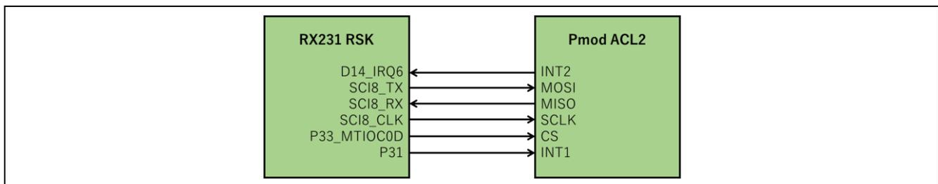
Figure 5-1 Hardware Block Diagram
