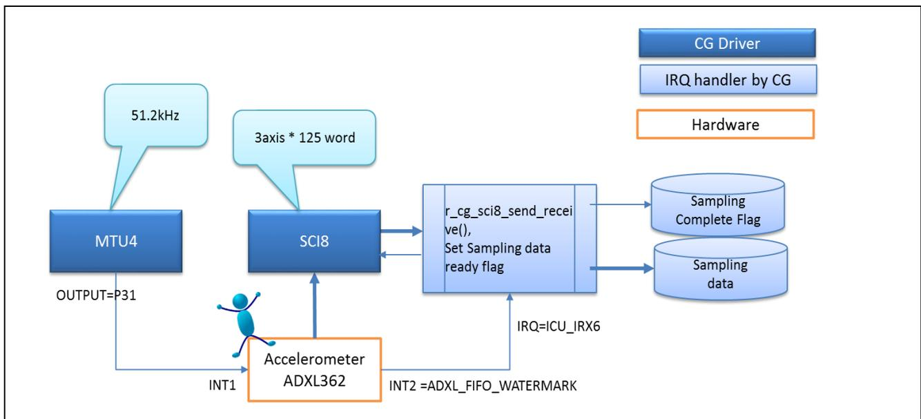
Figure 5-3 Respiratory Rate Measuring Digital Interconnect
