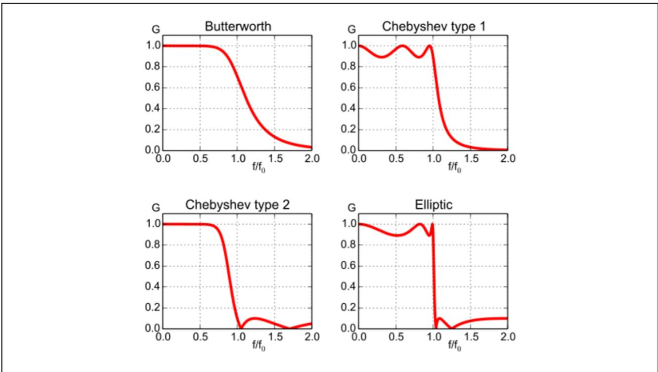
Figure 3-2 Gain distribution of discrete-time filters
