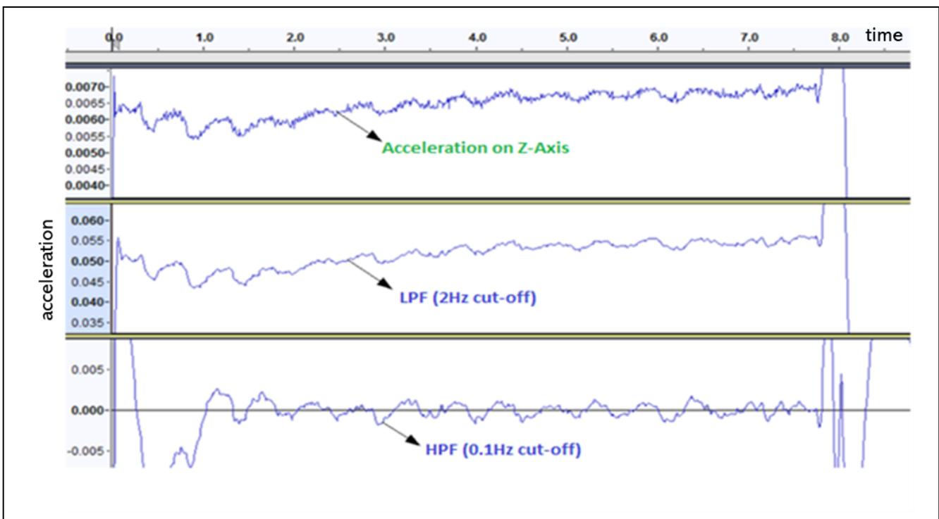
**Figure 3-3 Acceleration samples representation**
