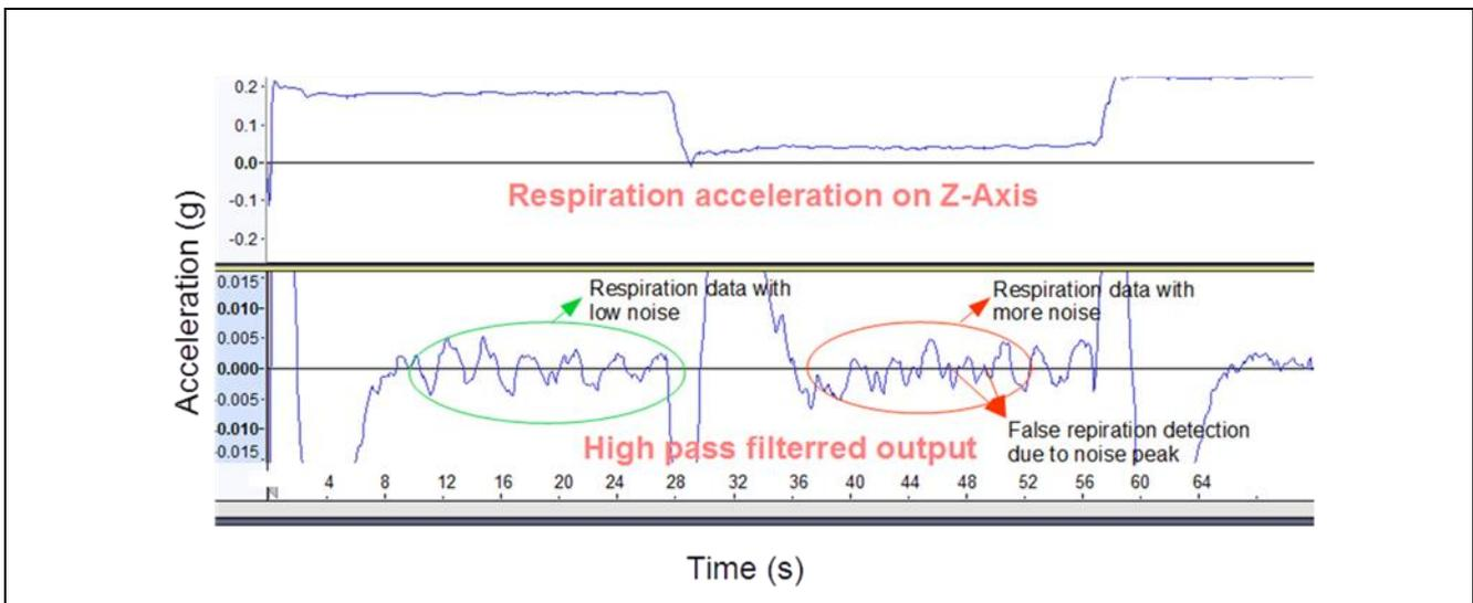
**Figure 3-4 False respiration detection due to noise peaks**
