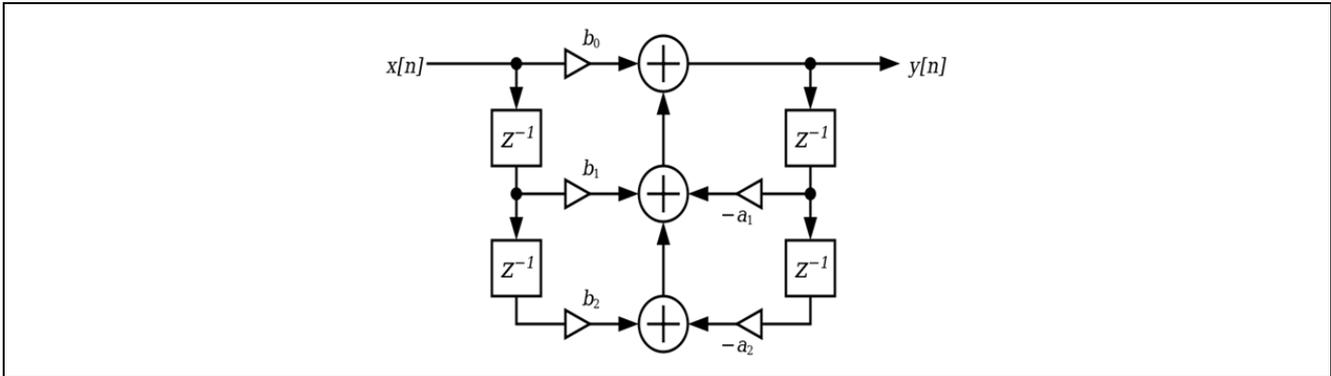
Figure 3-1 Flow graph of Biquad filter (Direct Form 1)
