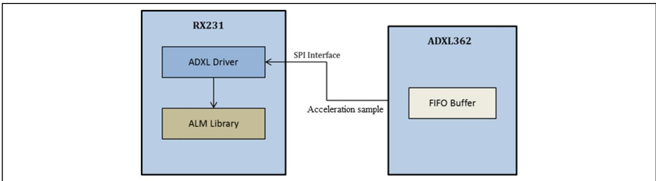
Figure 5-3 Interface of the ADXL362 Sensor with the MCU
