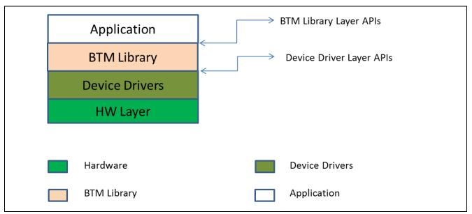
Figure 5-4 BTM Software Architecture
