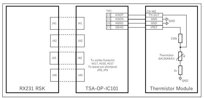
Figure 5-2 Hardware Wiring Chart
