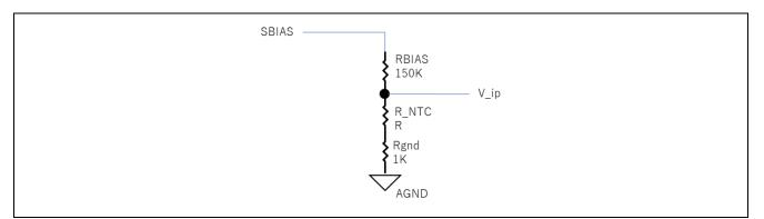
Figure 3-1 Body Surface Temperature Measurement Circuit
