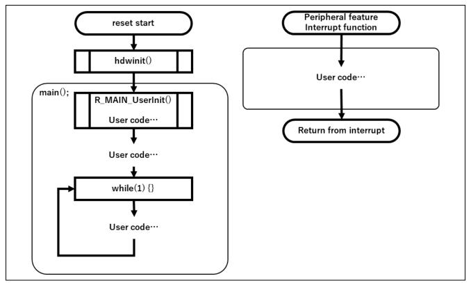
Figure 5-7 Application Framework by the Code Generator
