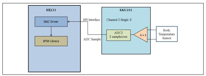
Figure 5-5 Interfacing of the Body Surface Temperature Sensor with the MCU via SAIC101
