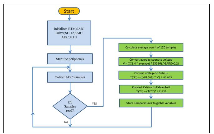
Figure 5-6 BTM Software Control Flow
