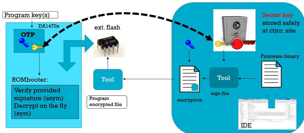
**Figure 1: Asymmetric Crypto for Bootloading**
