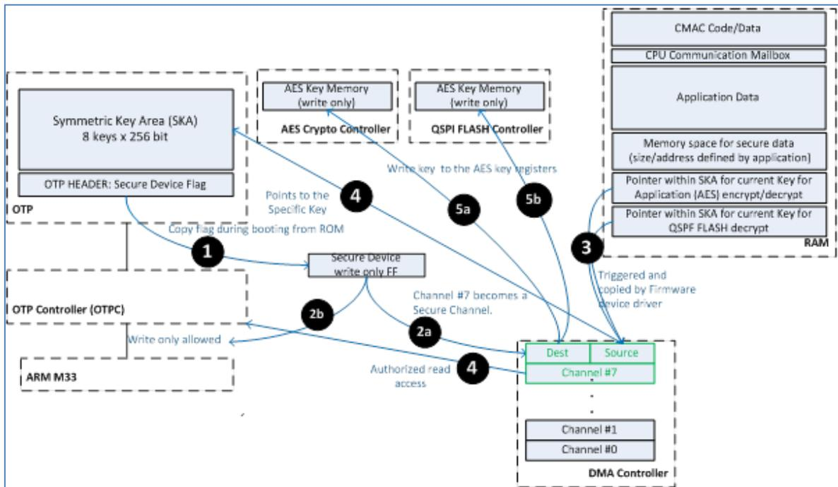
**Figure 4: Secure DMA Engine**
