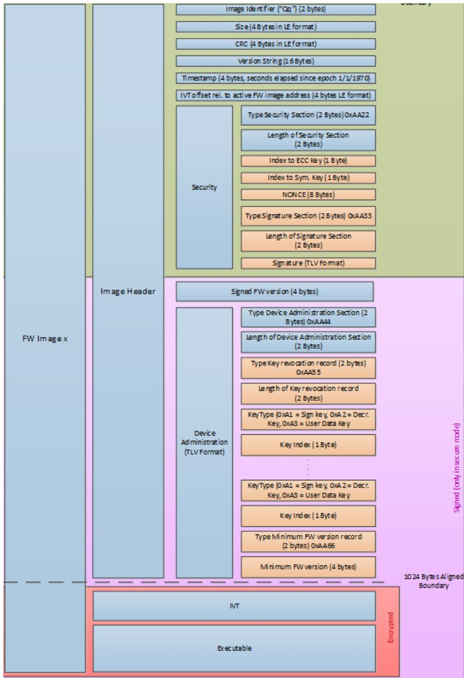
Figure 7: DA1470x Firmware Image Including Image Header
