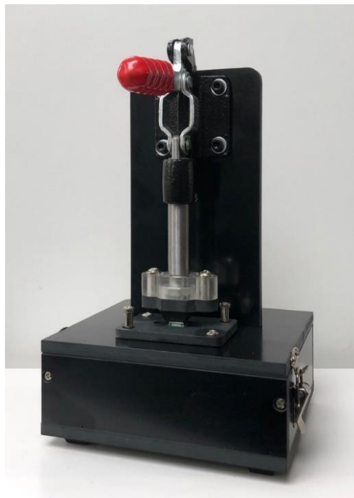
Figure 1: Photo of the DA14531 Test Jig
