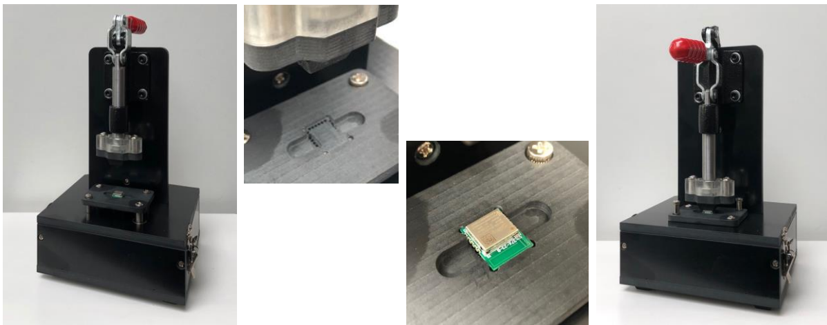
Figure 8: Opened Jig - Empty Module Holder - Module in Holder - Closed Jig
