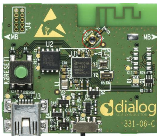
Figure 4: Pro-DK board, RF-connector J7
