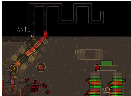
Figure 37: RF Matching Circuit must be Placed as Close as Possible to the Antenna
