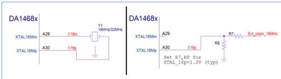
Figure 14: Connection of the crystal (left) and external 16 MHz clock (right) for AQFN package
