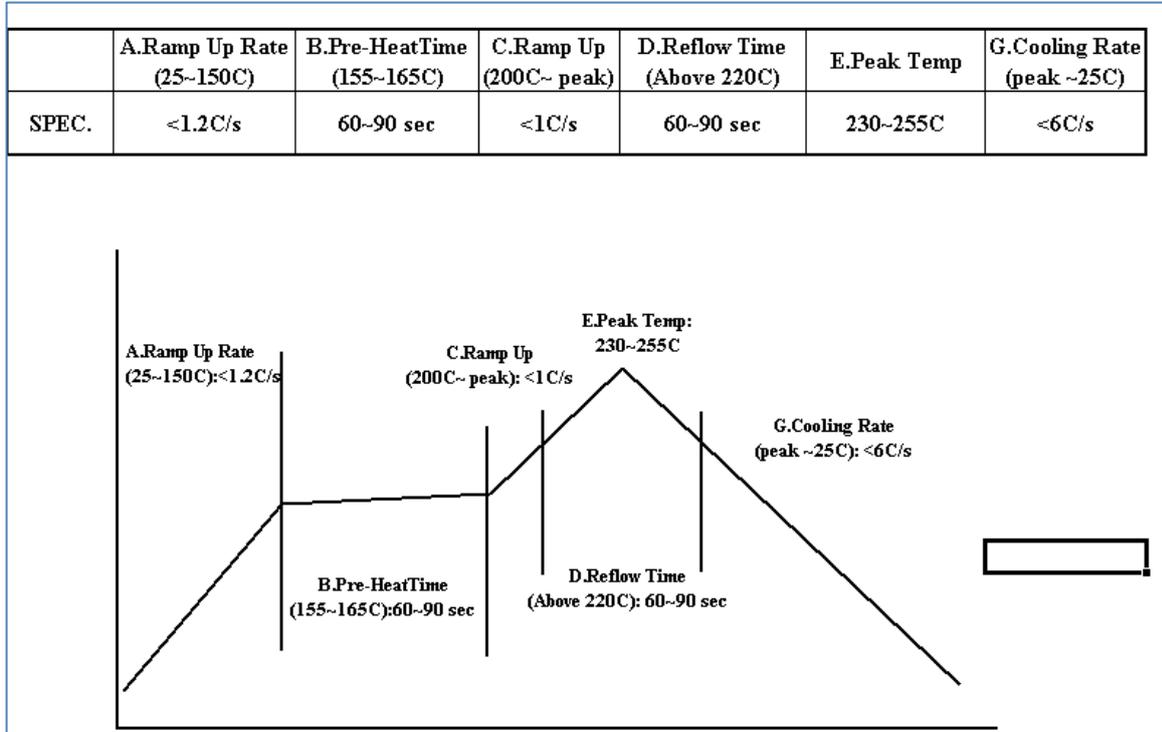
Figure 37: Reflow profile for solder paste SAC305
