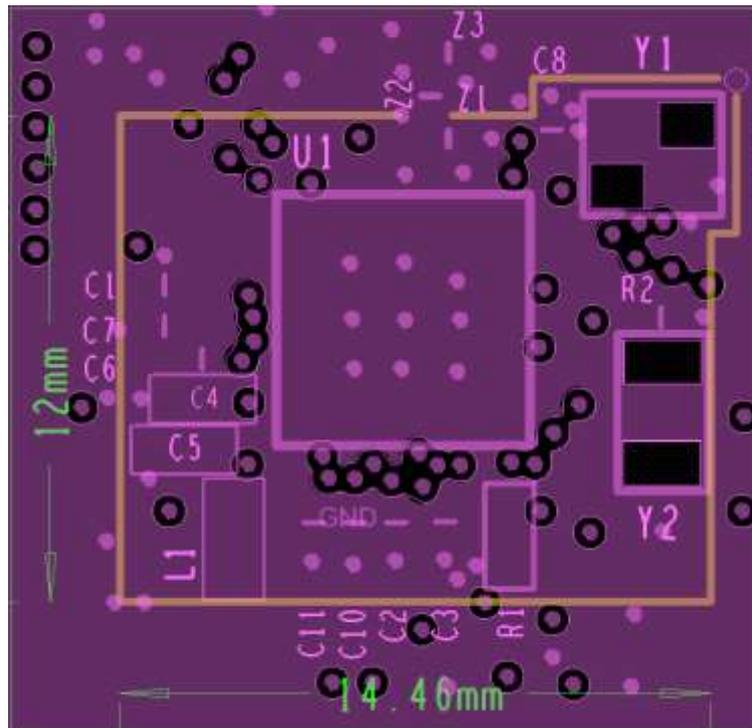
Figure 34: AQFN60 PCB layout, layer2, reference ground
