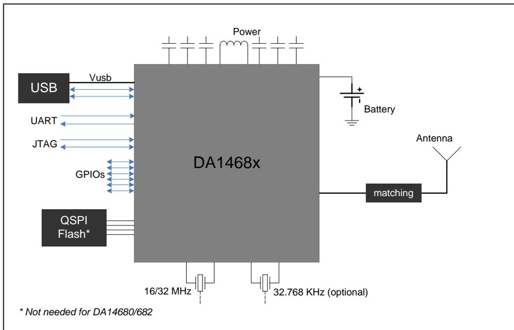
Figure 1: Block diagram of the DA1468x minimal design
