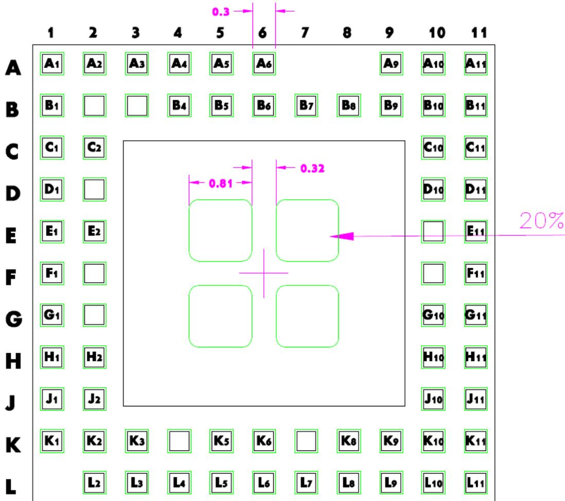
Figure 36: Recommend of stencil opening of thermal
