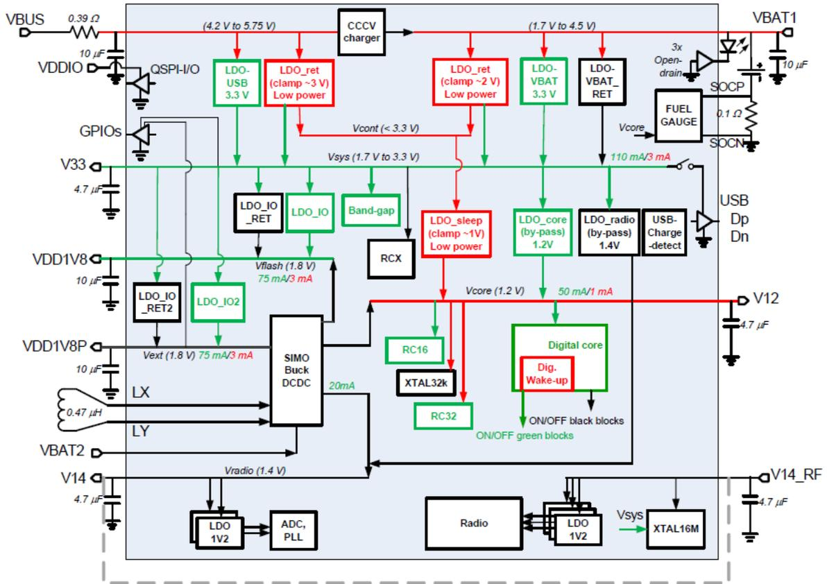
Figure 8: DA1468x power management unit block diagram
