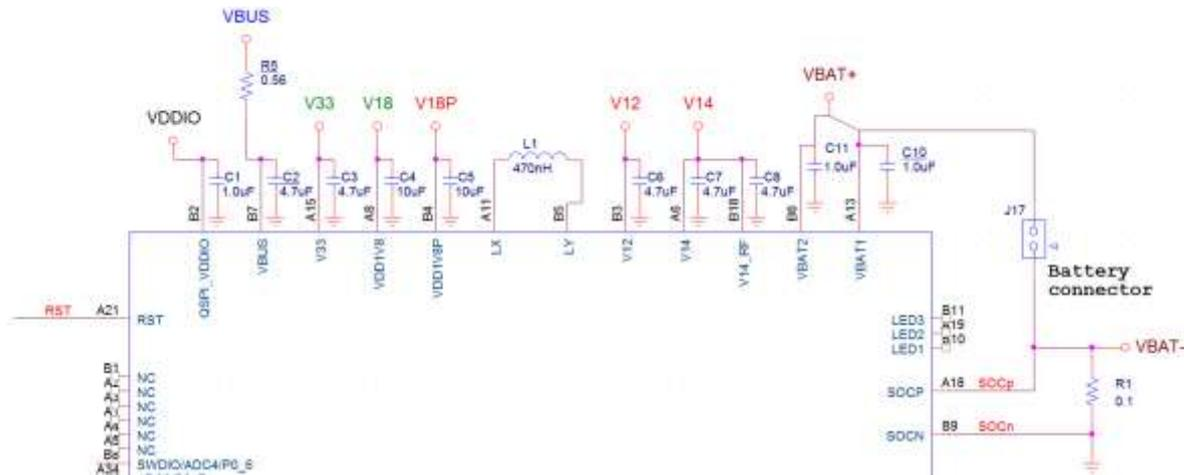
**Figure 6: The power section of the DA1468x**
