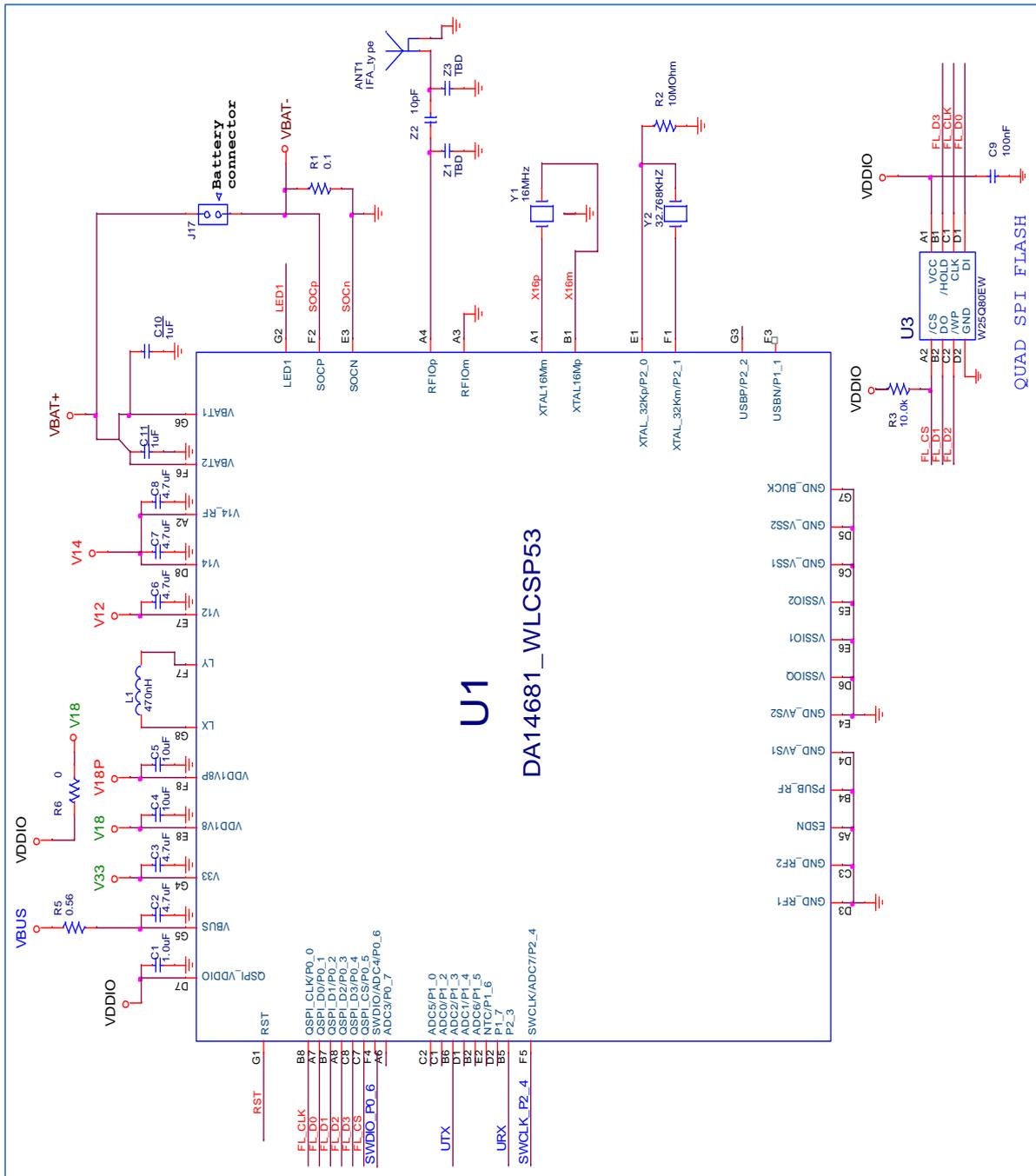
Figure 4: Minimal design for DA14683-00 WLCSP53 package
