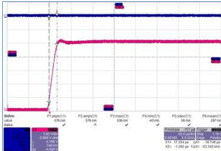
**Figure 23: Step response of VBUS with 0.39 Ω and 10 μF for a 1.5 m USB cable.**
