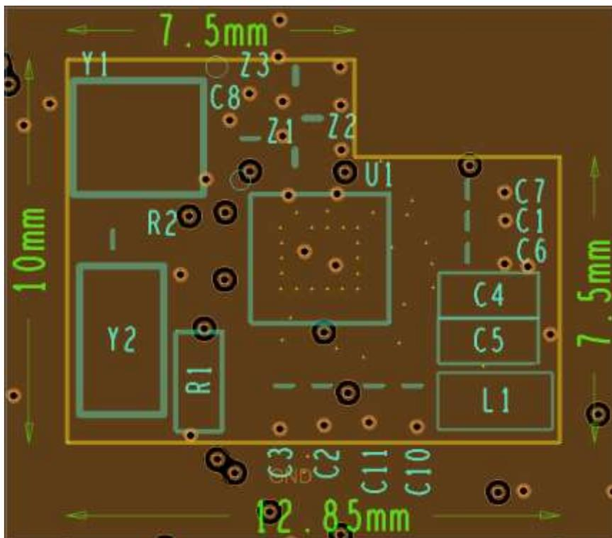
Figure 30: WLCSP53 PCB layout, layer 3, reference GND
