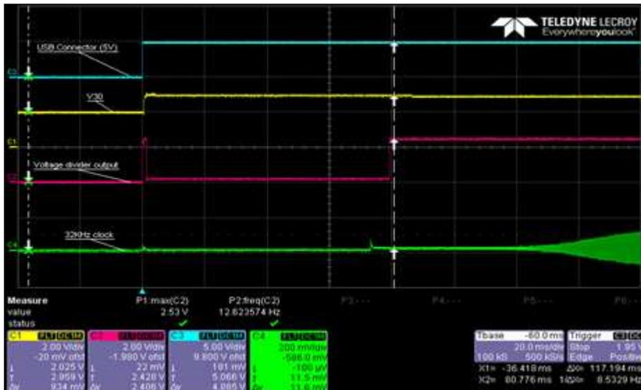
Figure 25: GPIO set as Input (no pull)
