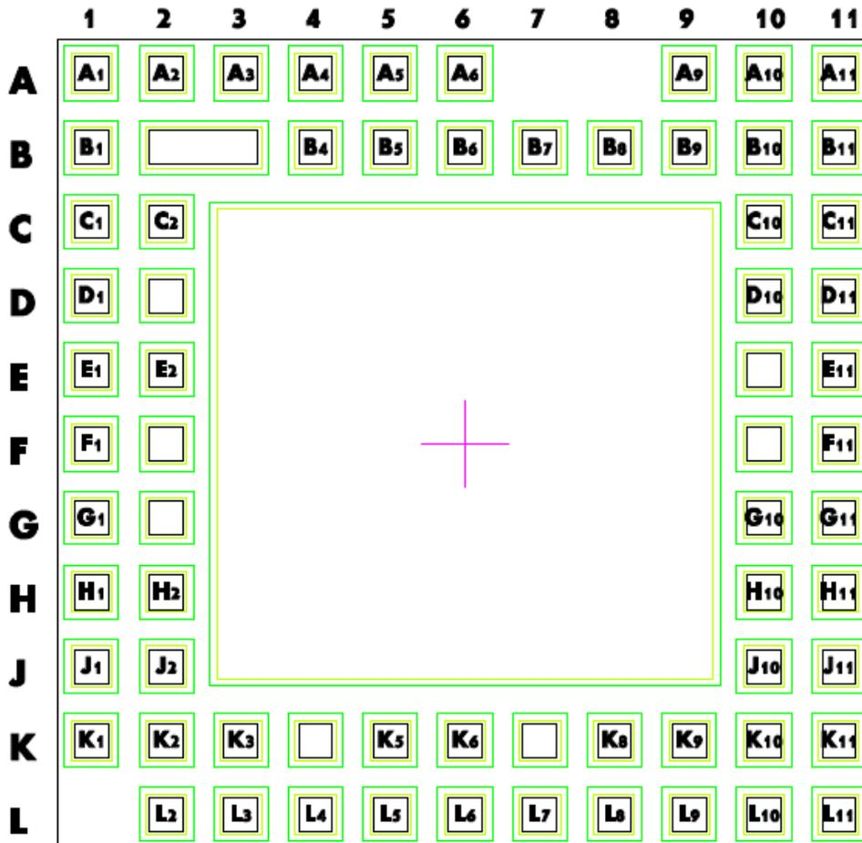
Figure 35: PCB footprint data
