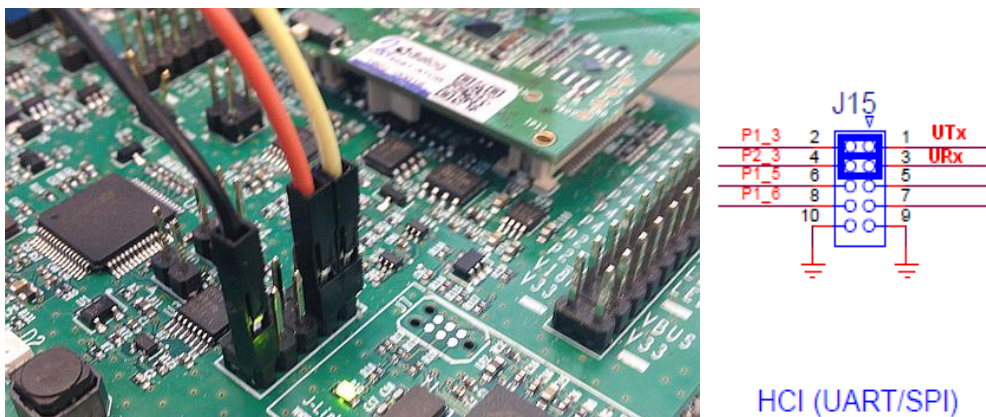
Figure 5: UART connection at Pro-DK J15
