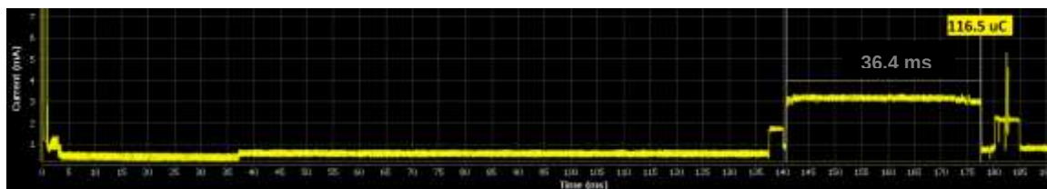
Figure 11: SPI memory mirroring into SRAM (with secondary bootloader)
