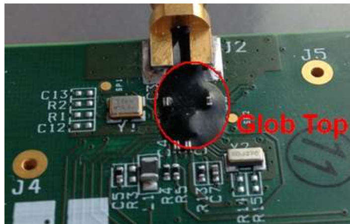
Figure 1: A failing DA1458x board with a low viscosity epoxy type Glob Top
