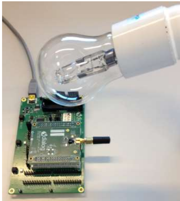
Figure 5: Halogen lamp test setup (10 cm above DA1458x board)
