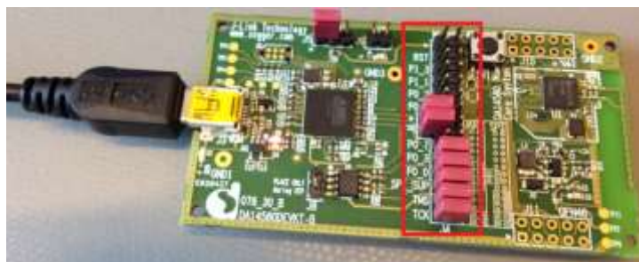
Figure 4: BASIC development HW configuration
