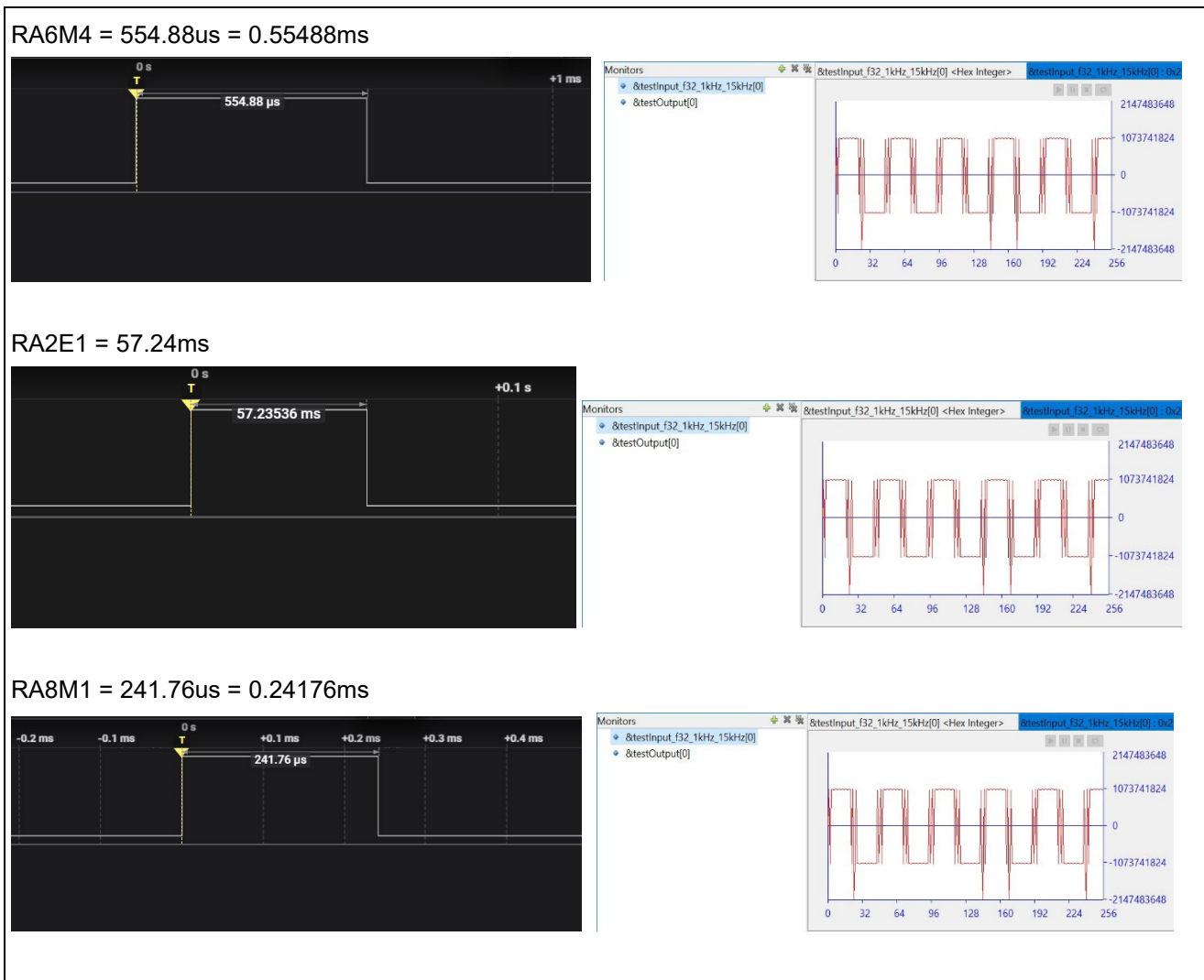
Figure 27. Timing measurement of EK-RA6M4, EK-RA2E1 and EK-RA8M1
