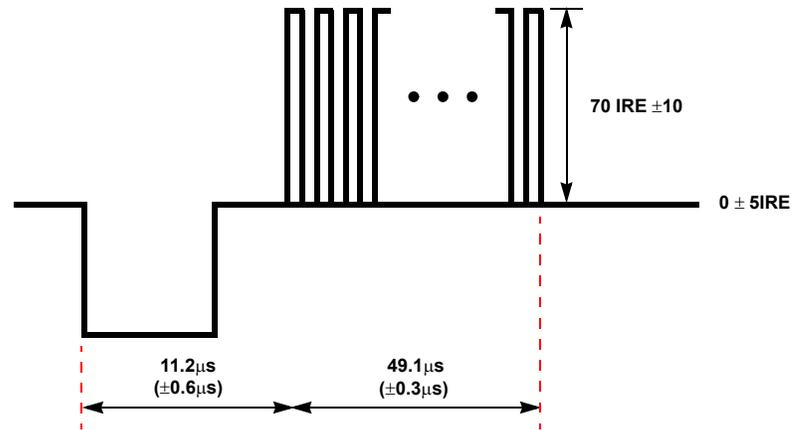
FIGURE 2. 525-LINE WSS LINE 20 AND LINE 283 TIMING
