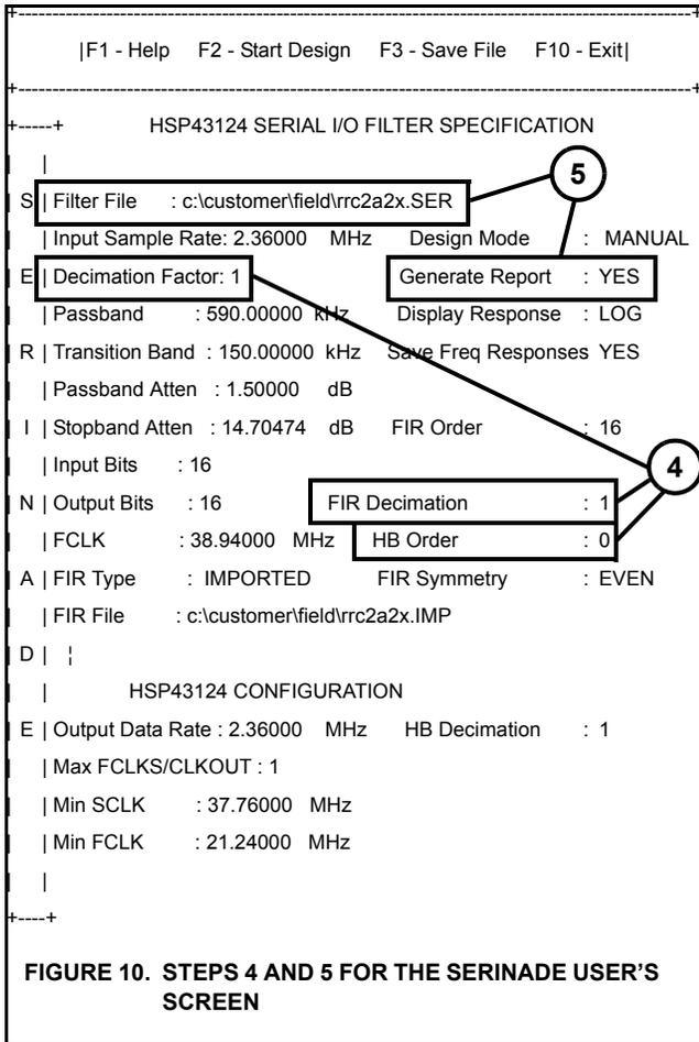
Hit F2, and the SERINADE software creates the proper filter report filer. Figure 11 shows the frequency response that is displayed on the screen.
