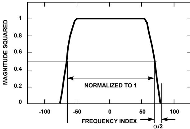
FIGURE 6. FREQUENCY RESPONSE OF AN IDEAL RRC
