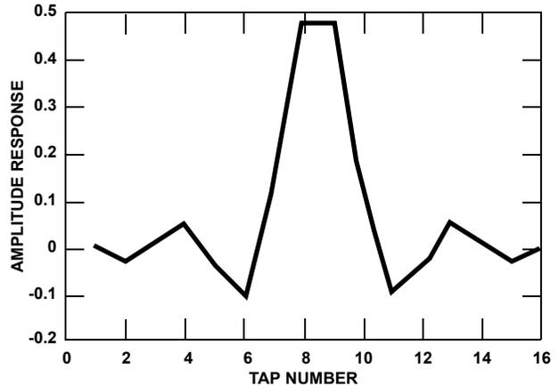
FIGURE 4. IMPULSE RESPONSE OF THE 16 TAP RRC FILTER
