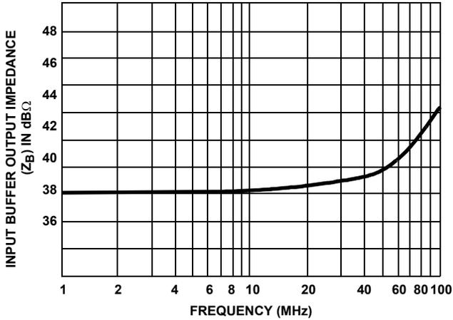
FIGURE 13. HA5020 INPUT BUFFER OUTPUT RESISTANCE vs FREQUENCY
