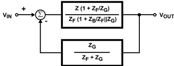
FIGURE 7. BLOCK DIAGRAM OF THE NON-INVERTING CFA
