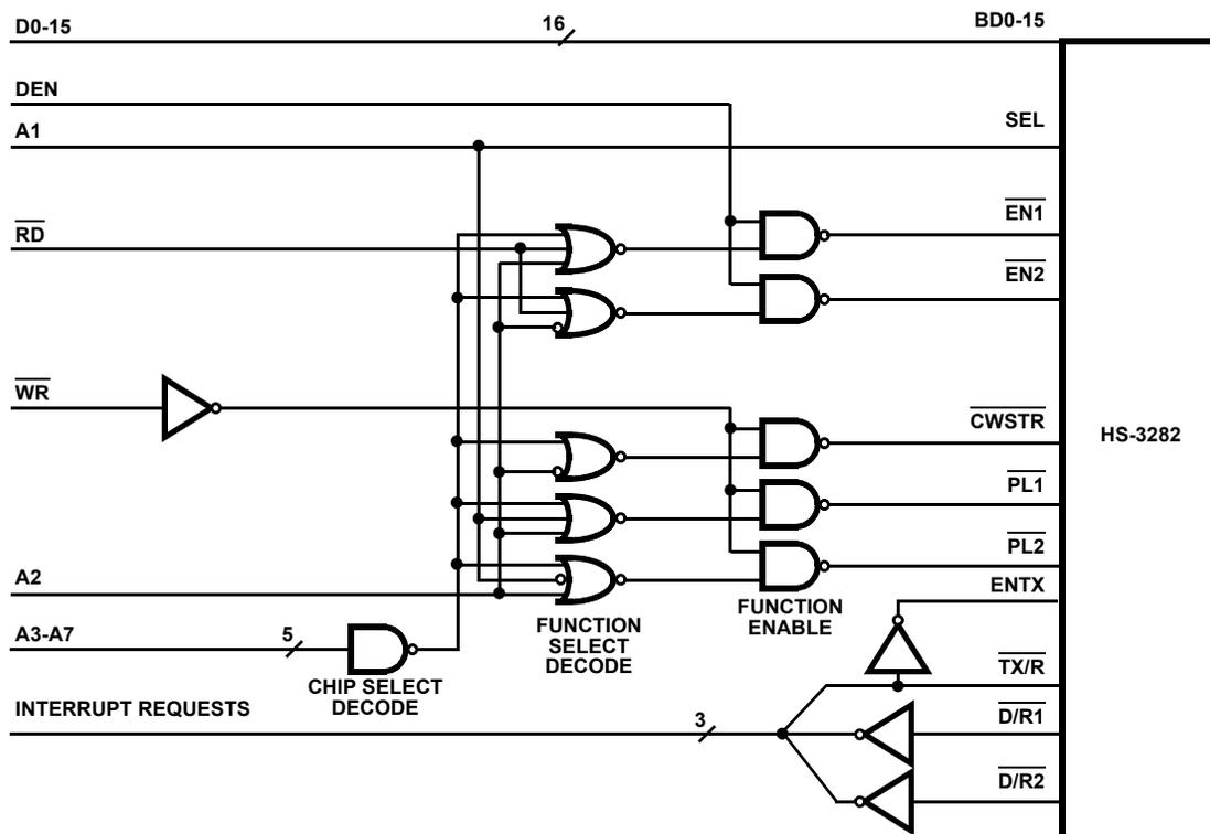
FIGURE 1. TYPICAL HOST TO HS-3282 INTERFACE LOGIC
