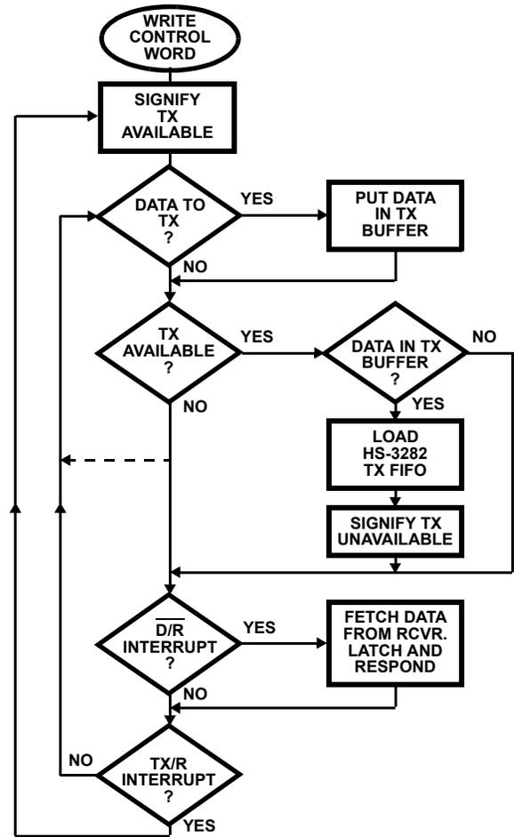
FIGURE 2. SIMPLE HS-3282 DRIVER ALGORITHM
