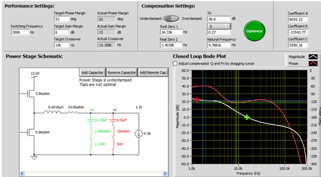
**Figure 7. CompZL Manual Results, with Mid-Band Gain Boost**
