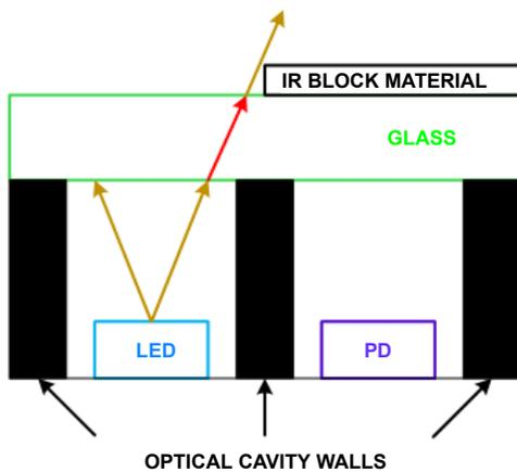
FIGURE 2. LIGHT PATH WITH ONLY THE PD COVERED
