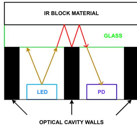
FIGURE 1. REFLECTIONS WITH COVERED EMITTER AND PD
