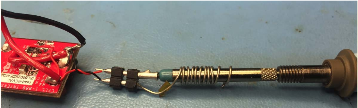
FIGURE 14. CONNECTION USING NEW HIGH FREQUENCY INTERCONNECT METHOD
