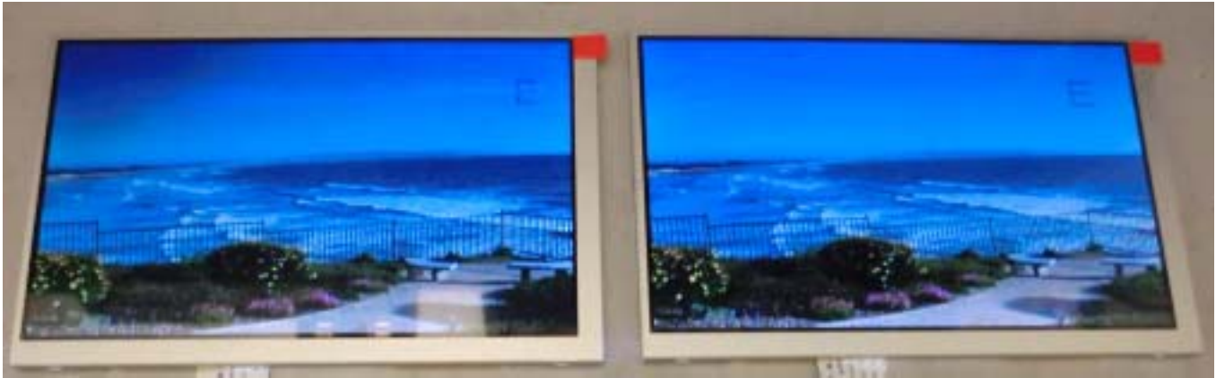
FIGURE 1. DUAL LCD SCREEN DRIVEN BY A COMMON VIDEO SIGNAL
